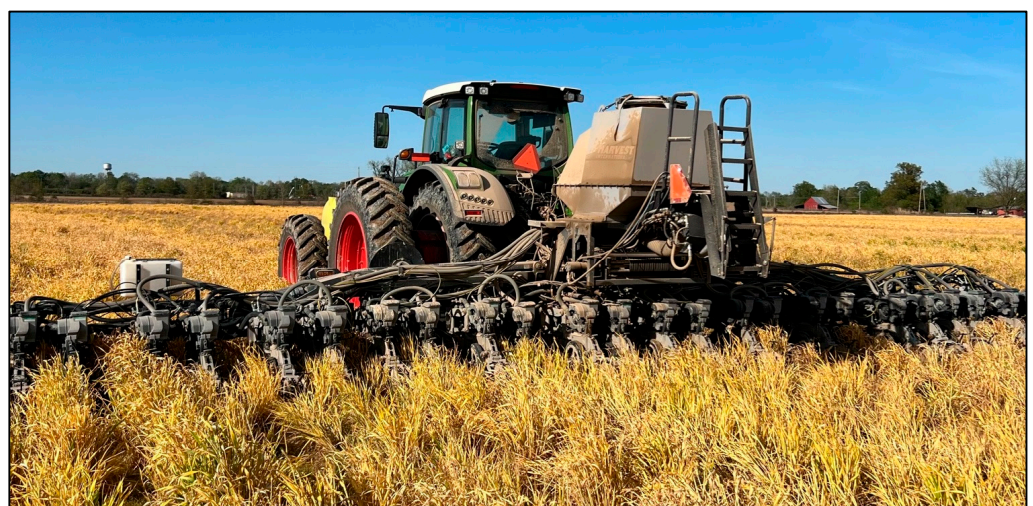
Figure 2. Tractor-mounted direct-seeder for large-scale establishment of SRI rice in Arkansas, USA, designed to plant seeds with SRI spacing through a cover crop or the residue of a previous rice crop. (Picture courtesy of Adam Chappell).
