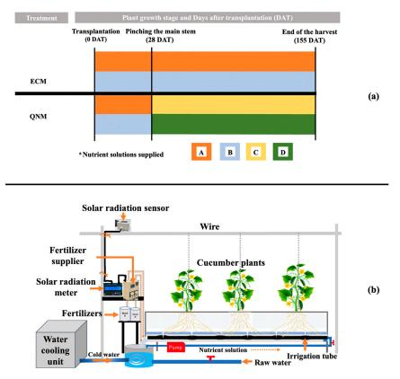
**Figure 1.** Nutrient solution supply scheme (**a**) and schematic diagram of the cultivation system (**b**). <sup>a</sup> The details of the nutrient solutions are in Table 1.
