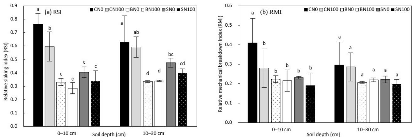
**Figure 3.** (a,b) Soil aggregate relative slaking index and relative mechanical breakdown index in different soil depths. Note: RSI is the stability of aggregate under the slaking of air under pressure in the pores of moist soil; RMI is the stability of aggregate under external stress.
