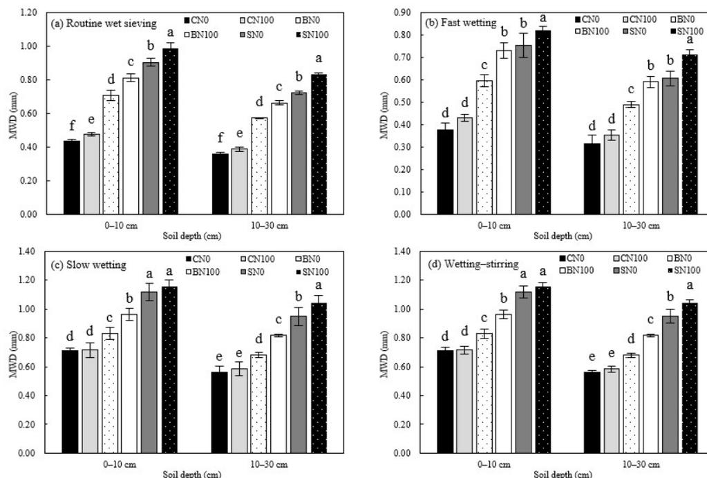
**Figure 2.** (a–d) Soil aggregate MWDs in different soil depths by using different sieving methods (mm). Note: Small letters in the same soil depth denote significant differences among the various treatments at  $p \leq 0.05$ , the same below.
