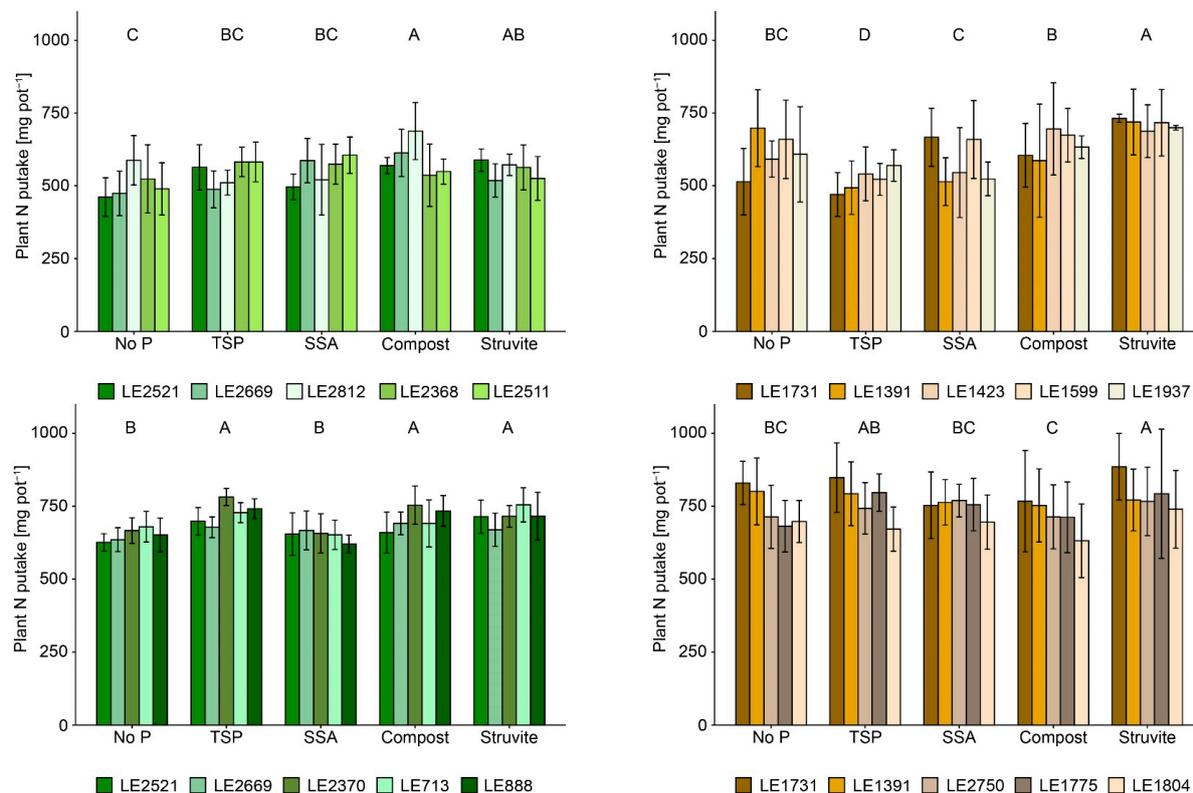
**Figure 3.** Plant nitrogen (N) uptake of alfalfa and red clover accessions in the five treatments (no P, TSP, SSA, compost and struvite) in PE1 (upper part) and PE2 (lower part). Different shades of green and brown colours are illustrated to differentiate between alfalfa and red clover accessions, respectively. Letters denote significant differences among treatments (using the means of accessions) (Duncan’s new multiple-range test, with  $p < 0.05$ ,  $n = 4$ ).
