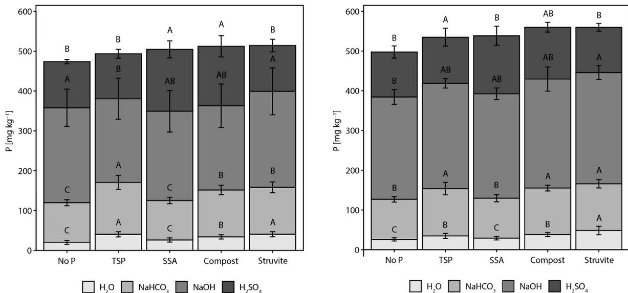
**Figure 5.** Phosphorus (P) concentrations of P-H<sub>2</sub>O, P-NaHCO<sub>3</sub>, P-NaOH and P-H<sub>2</sub>SO<sub>4</sub> in soil of five treatments (no P, TSP, SSA, compost, and struvite) for alfalfa (**left**) and red clover (**right**) in PE1. Letters denote significant difference between treatments (in means of accessions) (Duncan’s new multiple-range test, with  $p < 0.05$ ,  $n = 8$ ).
