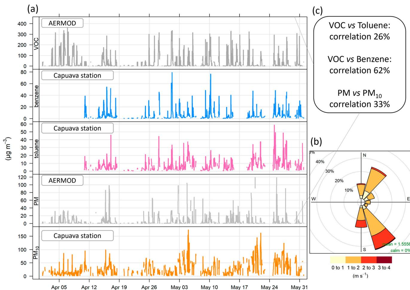
**Figure 6.** (a) Hourly mean concentrations for benzene, toluene, and  $\text{PM}_{10}$  at Capuava AQS, VOC, and PM (AERMOD: modeled data) during the episode (April to May 2021), white spaces are missing values. (b) The wind rose shows the wind speed ( $\text{m s}^{-1}$ ) and wind direction ( $^\circ$ ), data were filtered by the preferential wind direction from the Capuava Petrochemical Complex ( $0^\circ$  to  $180^\circ$ ) (c) “Correlation” is the correlation coefficient of Pearson.
