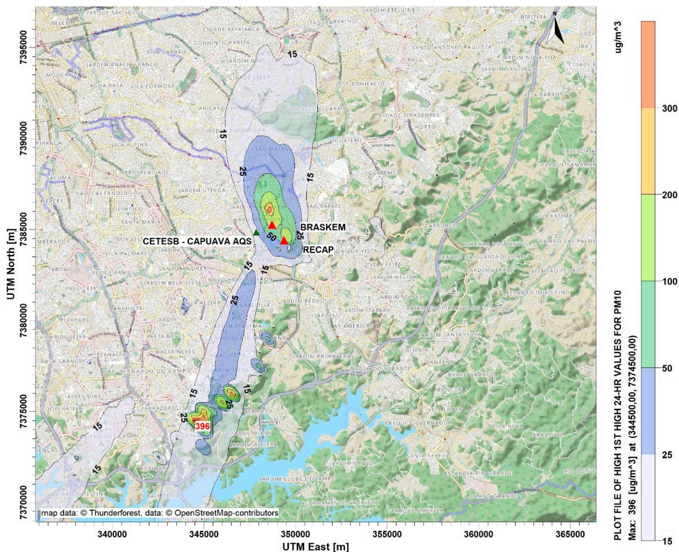
**Figure 8.** The maximum concentration of 24 h average ( $\mu\text{g m}^{-3}$ ) of PM in the affected area during the CPC maintenance period.
