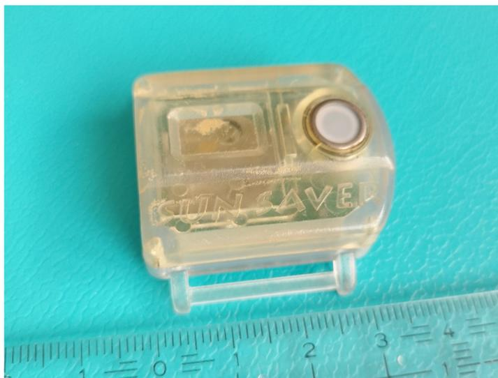
**Figure 1.** Electronic miniature UV-meter of the Sunsaver type [27].
