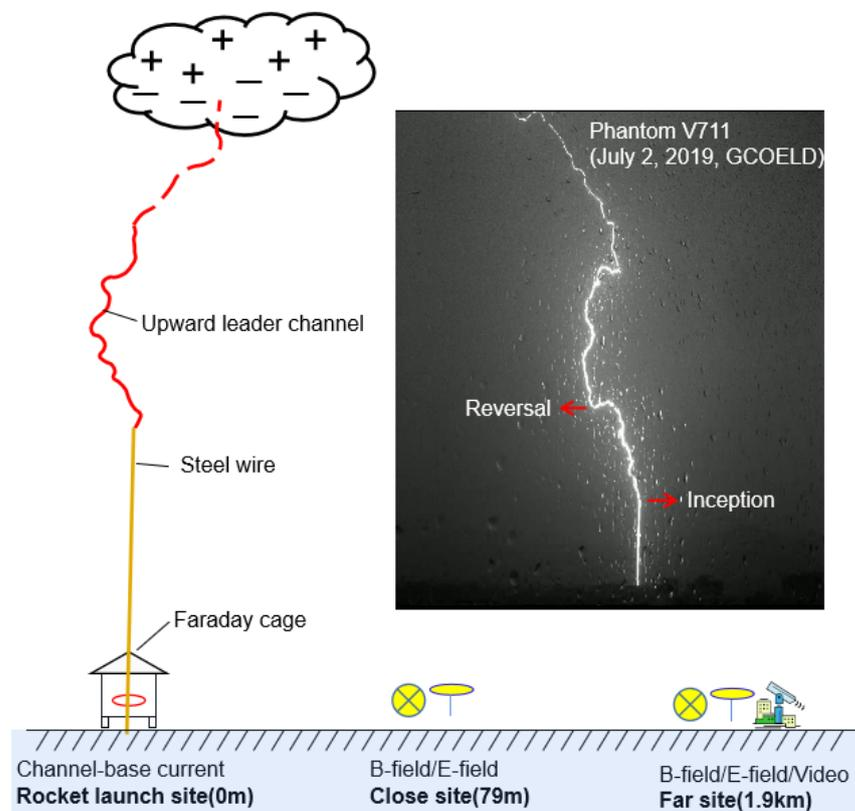
**Figure 3.** Schematic diagram of the initial process of triggering lightning with a wired rocket during the triggered lightning experiment: Field Experiment Base on Lightning Sciences, China Meteorological Administration [44]. The symbol + represents positive charge, and the symbol – represents negative charge.
