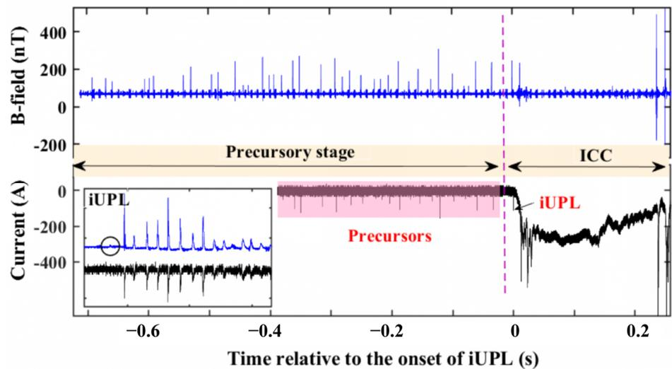
**Figure 12.** Channel-base current waveform (black line) and close B-field signals (blue line) at the triggered site, during the precursory stage of negative rocket-triggered lightning flashes (self-drawing).
