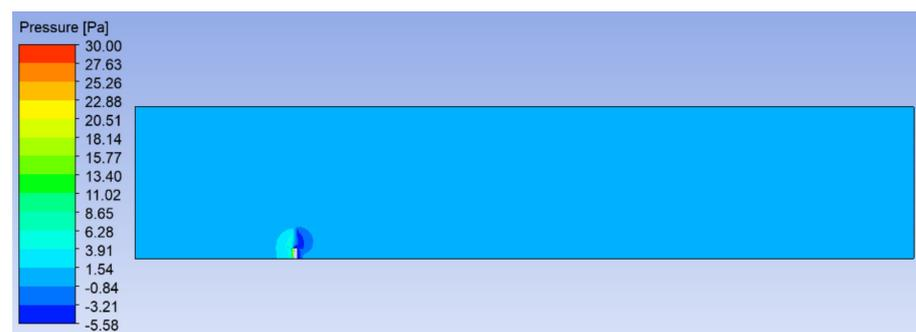
**Figure 5.** The pressure distribution in the vertical plane at  $y = 0$ .
