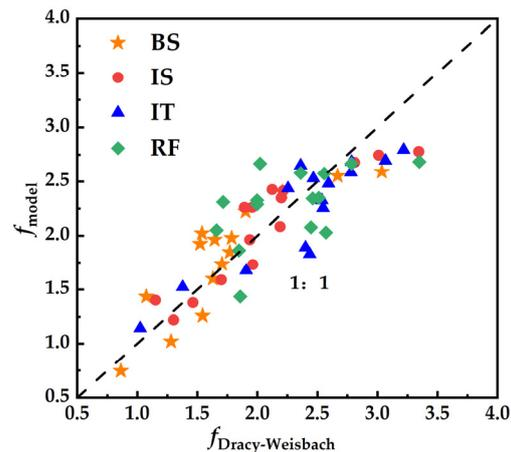
**Figure 12.** Comparison of the Darcy–Weisbach drag coefficients with those predicted using Equation (23).
