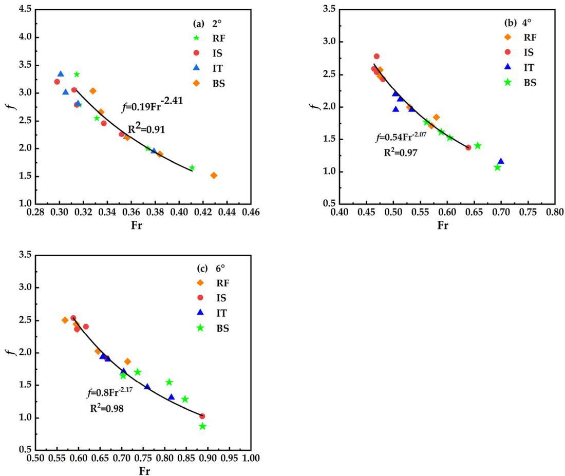
Figure 11. Plots of Froude number versus drag coefficient for slopes of 2° (a), 4° (b), and 6° (c) sequentially.
