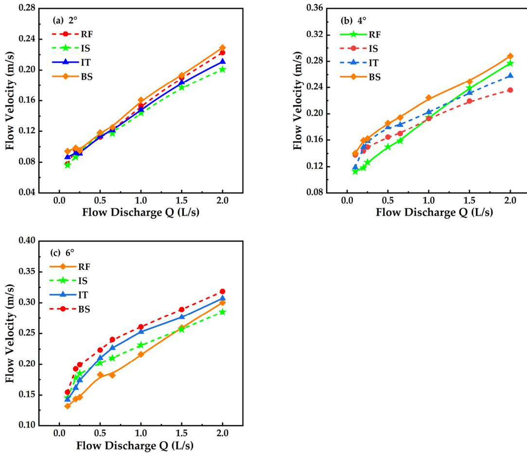
**Figure 6.** Plots of flow rate versus flow velocity for slopes of 2° (a), 4° (b), and 6° (c).
