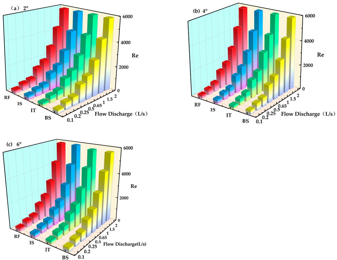
**Figure 7.** Flow versus Reynolds number, in order of slope 2° (a), 4° (b), and 6° (c).
