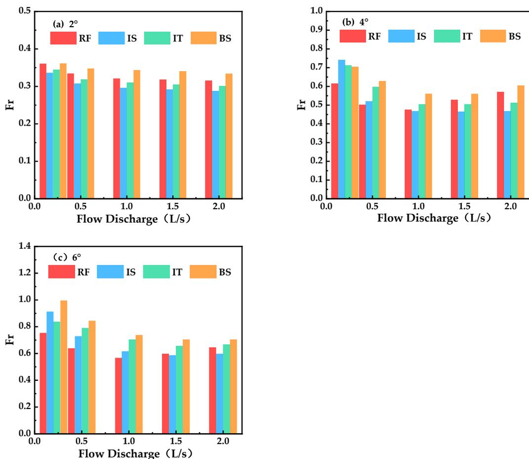
**Figure 8.** Flow rate versus Froude number for slopes of 2° (a), 4° (b), and 6° (c), in this order.
