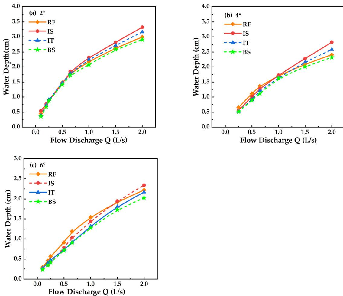
**Figure 5.** Plot of discharge versus water depth at different gradients in order of gradient 2° (a), 4° (b), and 6° (c).
