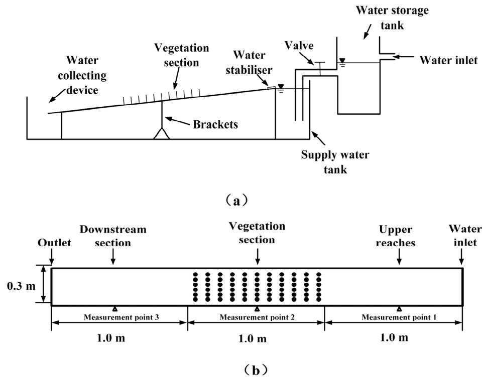
Figure 2. Diagram of the test setup (a); diagram of the test configuration (b).
