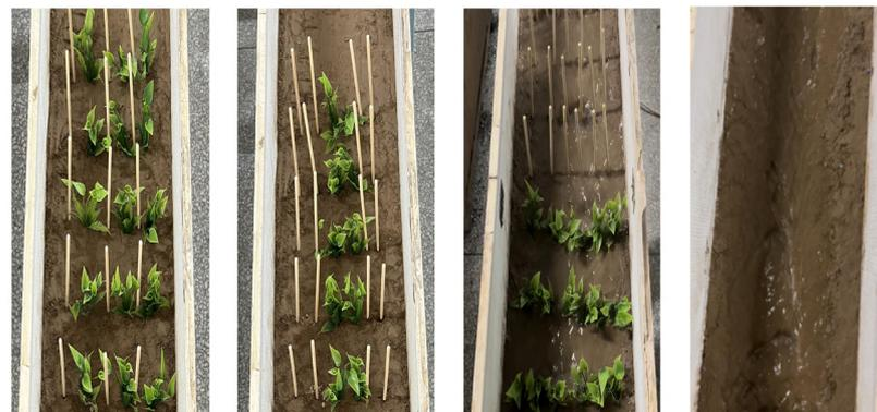
(a) Rigid flexible interspersed in a single row (b) Rigid flexible interspersed in two rows (c) Rigid upstream and flexible downstream (d) Bare slope
