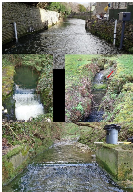
Figure 4. The surface water measurement sites. Top image is Peakshole Water (PW). The grey box on the right is a telemetric depth recorder installed by the Environment Agency in January 2024. The white vertical pipe houses the Odyssey capacitive water level logger. The stage board is on left wall and the weir is immediately downstream. Middle left is Russet Well (RW) and middle right is Slop Moll (SM), where the red arrow points to a pipe housing the Odyssey capacitive water level logger. Bottom image is the Peak Cavern Rising (PCR) weir. The vertical grey pipe on the right houses the Odyssey capacitive water level logger.
