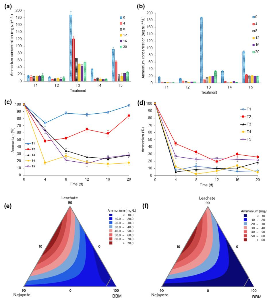
**Figure 3.** Ammonium removal profile in quantification for (a) *S. acutus* and (b) *H. pluvialis*. Ammonium removal profile in percentage (%) according to the initial value for (c) *S. acutus* and (d) *H. pluvialis*. Mixture contour plots in ammonium quantification for (e) *S. acutus* and (f) *H. pluvialis*.
