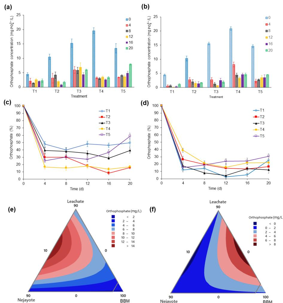
**Figure 4.** Orthophosphate removal profile in quantification for (a) *S. acutus* and (b) *H. pluvialis*. Orthophosphate removal profile in percentage (%) according to the initial value for (c) *S. acutus* and (d) *H. pluvialis*. Mixture contour plots in orthophosphate quantification for (e) *S. acutus* and (f) *H. pluvialis*.
