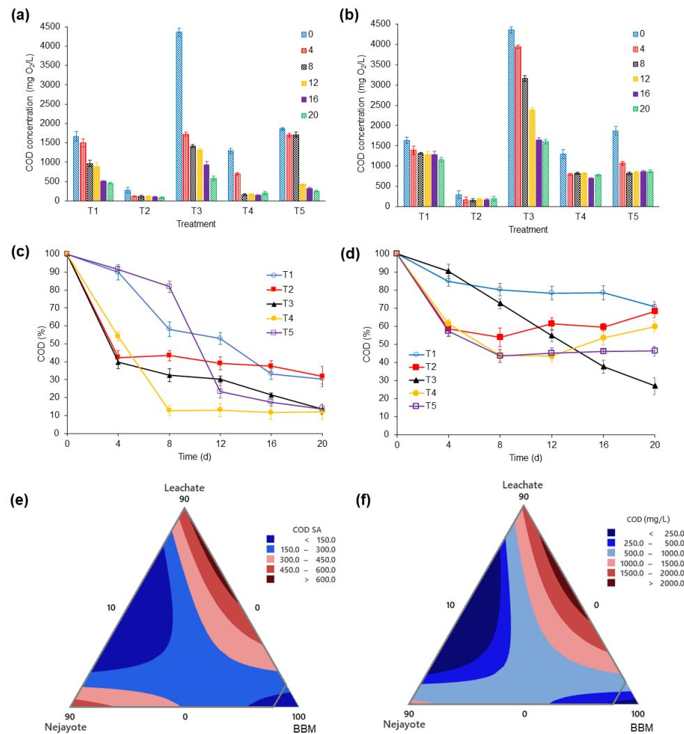
**Figure 5.** COD removal profile in quantification for (a) *S. acutus* and (b) *H. pluvialis*. COD removal profile in percentage (%) according to the initial value for (c) *S. acutus* and (d) *H. pluvialis*. Mixture contour plots in COD quantification for (e) *S. acutus* and (f) *H. pluvialis*.
