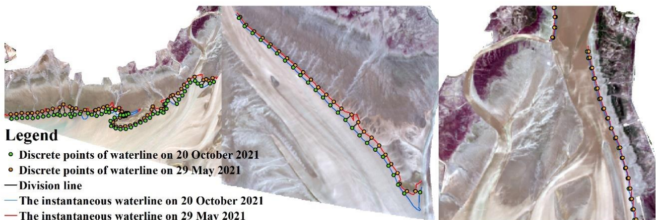
Figure 4. Tidal correction schematic diagram using instantaneous water edges.
