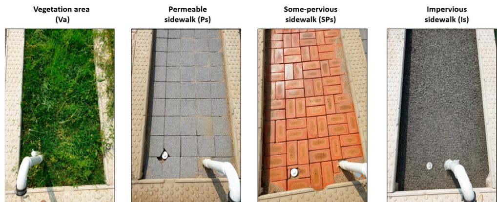
Figure 2. Classification of experiments according to 4 ground materials.
