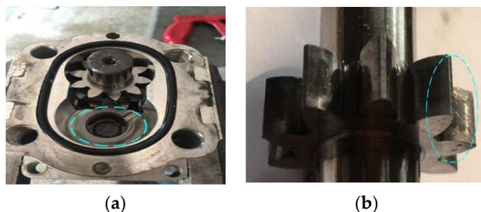
**Figure 6.** Wear and tear of gear pump: (a) side plate wear; (b) end-face wear of driving gear.
