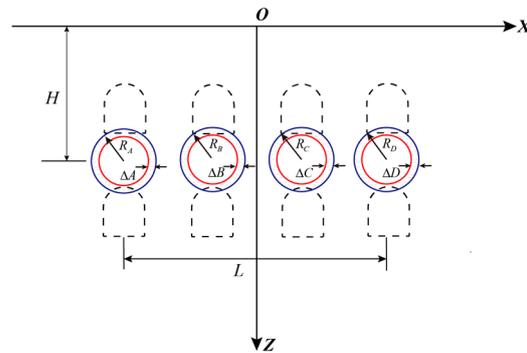
Figure 17. Equivalent pilot tunnels to circular tunnels.
