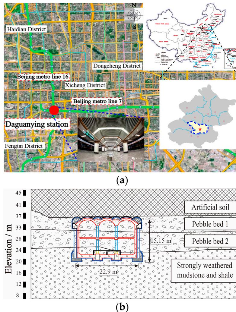
**Figure 1.** Daguanying subway station: (a) Location; (b) Structure profile.
