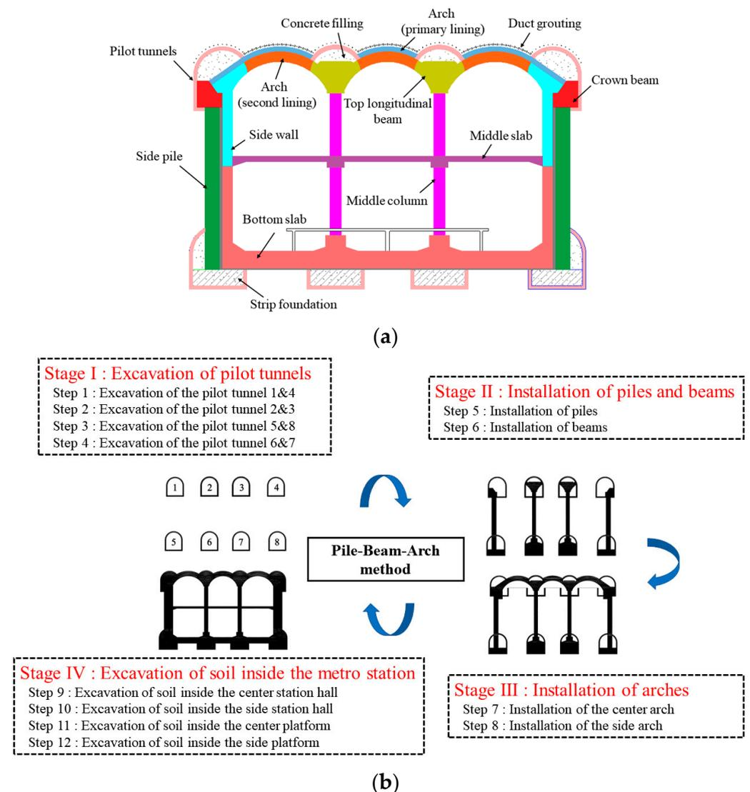
**Figure 2.** PBA method introduction: (a) structure composition; (b) Construction process.
