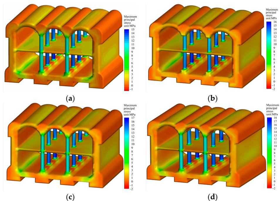
**Figure 14.** The maximum principal stress distribution of structure under different loads: (a)  $P = 20$  kPa; (b)  $P = 40$  kPa; (c)  $P = 60$  kPa; and (d)  $P = 80$  kPa.
