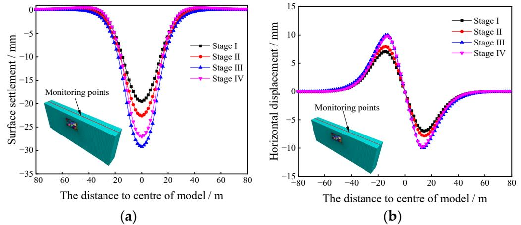
**Figure 5.** Surface displacement curves: (a) surface settlement; (b) surface horizontal displacement.
