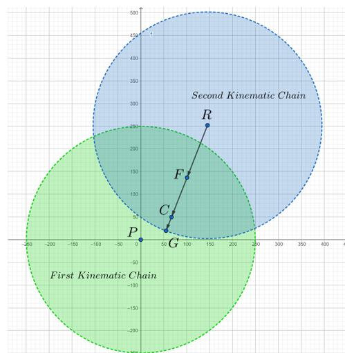
Figure 7. Robot’s workspace constraints due to both the first and second kinematic chain lengths.
