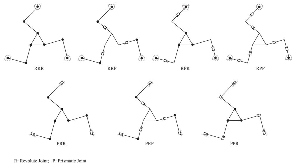
**Figure 1.** Possible parallel robots configurations.
