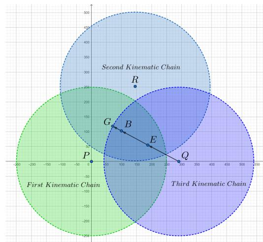
Figure 8. Robot’s workspace constraints due to all three kinematic chain constraints.
