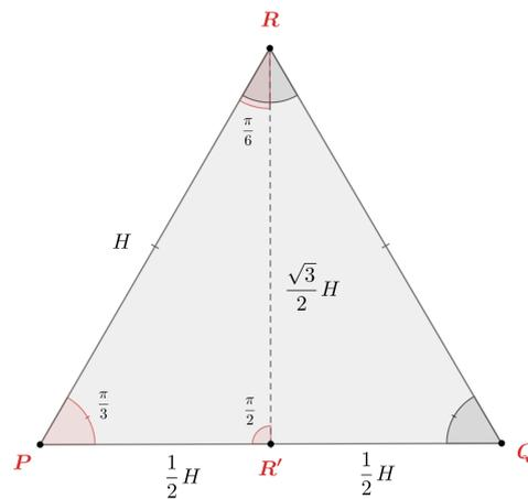
Figure 6. Planar parallel robot base joint positions.
