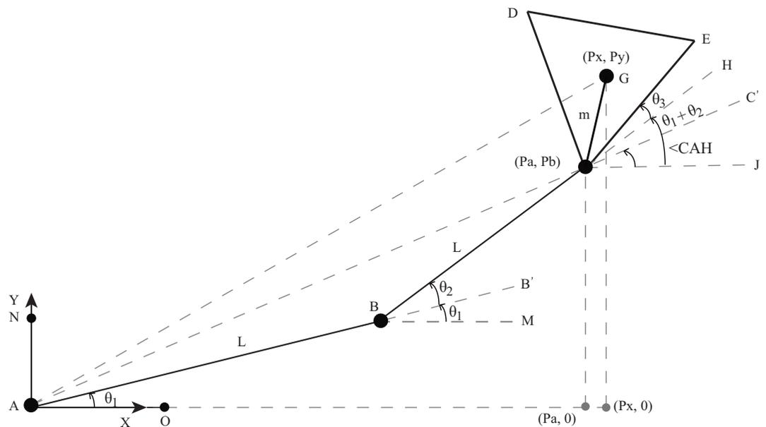
Figure 9. Kinematic chain geometry with active joints in A, B, and C.
