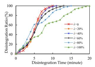
Figure 7. Relationship between disintegration ratio and time of mixed soil.
