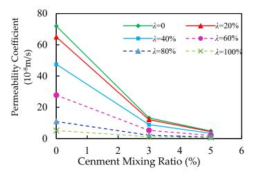
Figure 5. Variations of permeability coefficient with cement mixing ratio.
