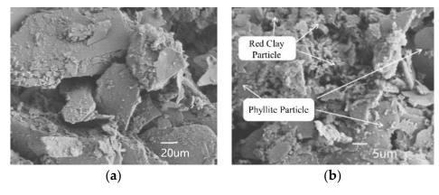
**Figure 13.** Microstructure of phyllite soil improved by red clay (a)  $\lambda = 0$  and (b)  $\lambda = 40\%$ .
