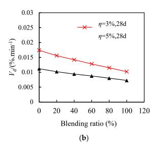
**Figure 10.** Disintegration rate vs blending ratio of red clay with different cement mixing ratio (**a**)  $\eta = 0$ ; (**b**)  $\eta = 3\%$  and  $\eta = 5\%$ .
