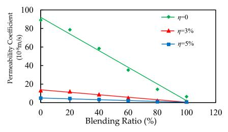
Figure 4. Variations of permeability coefficient with blending ratio of red clay.
