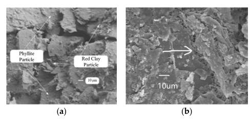
**Figure 14.** Network cementation of cement products between soil particles (a)  $\eta = 0$  and (b)  $\eta = 3\%$ .
