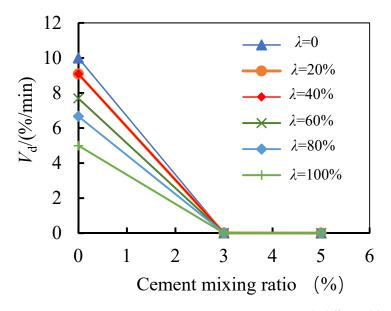
Figure 11. Disintegration rate vs cement mixing ratio with different blending ratios.
