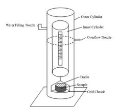
Figure 3. Sketch showing disintegration test apparatus.
