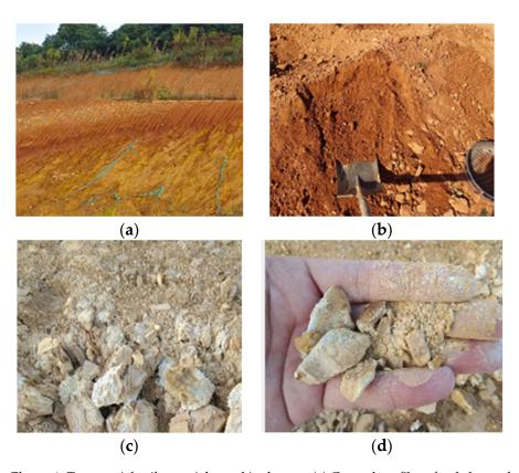
**Figure 1.** Two special soil materials used in the test. (a) General profiles of red clay and phyllite soils; (b) red clay stockpile; (c) close view of phyllite soil; (d) phyllite hardness.
