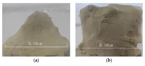
**Figure 6.** Comparison of disintegration process with and without cement. (a)  $\eta = 0$  (b)  $\eta = 3\%$ .
