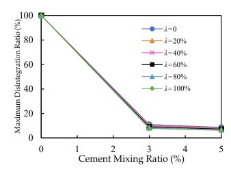
**Figure 9.** Variation rules of improved soil  $D_{\rm m}$  with cement mixing ratio.
