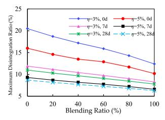
**Figure 8.** Relationship between  $D_{\rm m}$  and blending ratio of red clay with cement mixing ratios.
