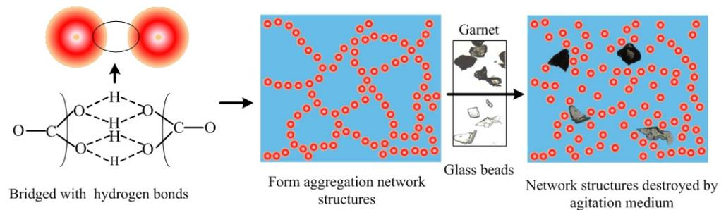
**Figure 3.** The interactions between fine calcite particles ( $\sim 20 \mu\text{m}$ ) in flotation slurry spiked with an agitation medium [118].
