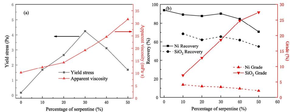
**Figure 2.** Effect of the percentage of serpentine on (a) rheological behaviors and (b) flotation performance of mixed minerals in the presence of PBX with a total pulp concentration of 40 wt% (pH = 9.5~10, PBX:  $1.5 \times 10^{-3}$  mol/L, MIBC: 100 mg/L) [59].
