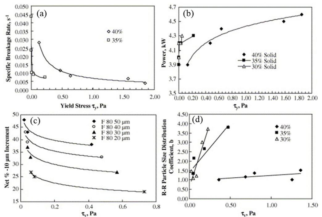
**Figure 1.** Specific breakage rate (a), agitator power (b), net production of  $-10 \mu\text{m}$  (c) and Rosin-Rammler particle size distribution coefficient (d) vs. pulp yield stress [26].
