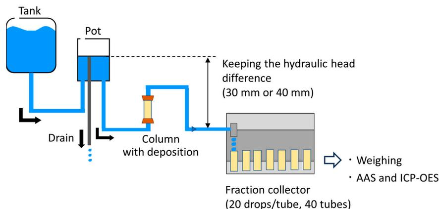
Figure 2. Schematic of flow experiment with overflow system.
