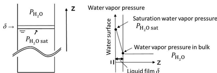
Figure 9. Conceptual diagram of water evaporation model.
