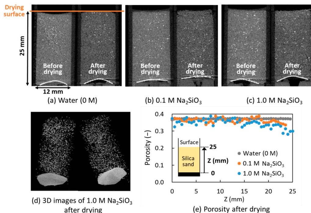
**Figure 8.** X-ray CT analysis for the SS columns filled with pure water and  $\text{Na}_2\text{SiO}_3$ . (a–c) Cross-sectional X-ray images before and after drying; (d) three-dimensional images for 1.0 M CsCl after drying; and (e) porosity after drying according to the height direction of the columns. The plots in (e) are average values of the porosity in the width direction at each height.
