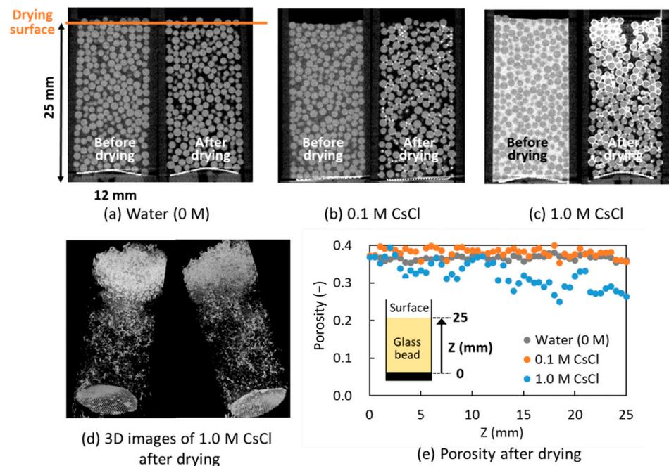
**Figure 5.** X-ray CT analysis of the GB  $\phi 1.0$  columns. (a–c) Cross-sectional X-ray images before and after drying; (d) three-dimensional images for 1.0 M CsCl after drying; and (e) porosity after drying according to the height direction of the columns. The plots in (e) are average values of porosity in the width direction at each height.
