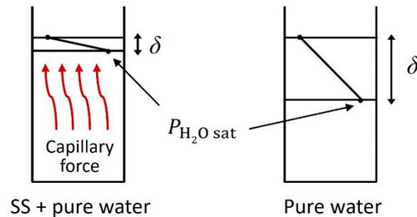
**Figure 11.** An image of the capillary force effect and liquid film thickness.
