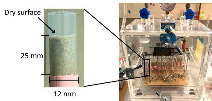
**Figure 1.** An image of the drying experiment in the vacuum desiccator containing silica gel.
