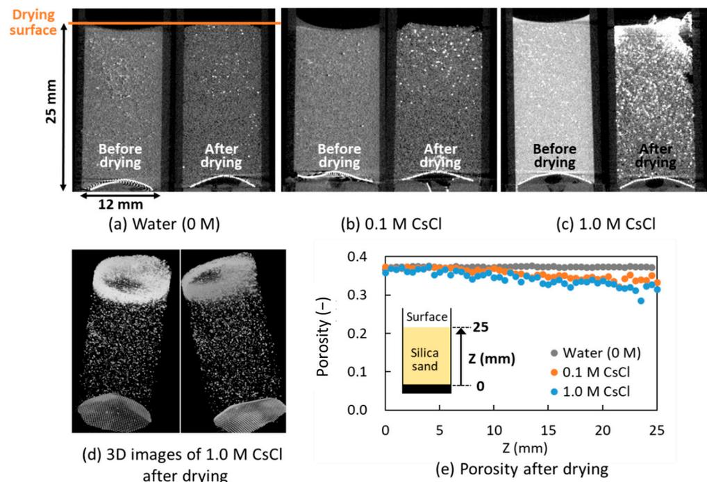
**Figure 7.** X-ray CT analysis for the SS columns filled with pure water and CsCl. (a–c) Cross-sectional X-ray images before and after drying; (d) three-dimensional images for 1.0 M CsCl after drying; and (e) porosity after drying according to the height direction of the columns. The plots in (e) are average values of the porosity in the width direction at each height.
