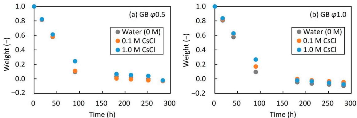
**Figure 3.** Weight change in the GB columns over time during the drying experiment ((a) GB  $\phi 0.5$ ; (b) GB  $\phi 1.0$ ). The vertical axis is normalized to the initial weight of the GB columns filled with solutions.
