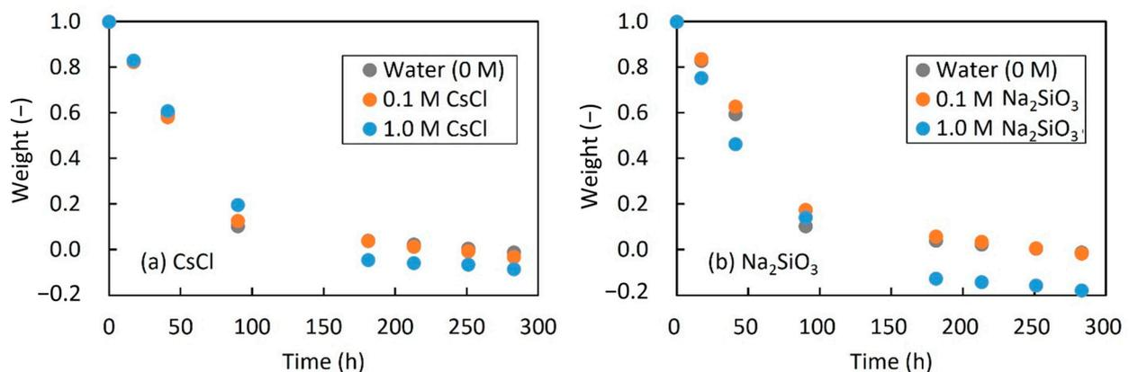
**Figure 6.** Weight change in the SS columns over time during the drying experiment ((a) CsCl; (b) Na<sub>2</sub>SiO<sub>3</sub>). The vertical axis is normalized to the initial weight of the SS columns filled with solution.
