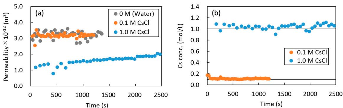
**Figure 12.** Changes in (a) permeability and (b) Cs concentration of the effluent over time for the SS columns with CsCl precipitation. The black lines in (b) indicate the Cs concentration in the influent.
