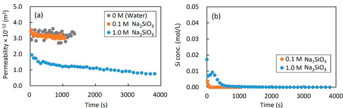
**Figure 13.** Changes in (a) permeability and (b) Si concentration of the effluent over time for the SS columns with Na<sub>2</sub>SiO<sub>3</sub> precipitation.
