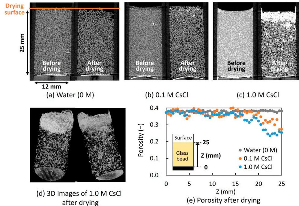
**Figure 4.** X-ray CT analysis of the GB  $\phi 0.5$  columns. (a–c) Cross-sectional X-ray images before and after drying; (d) three-dimensional images for 1.0 M CsCl after drying; and (e) porosity after drying according to the height direction of the columns. The plots in (e) are average values of the porosity in the width direction at each height.
