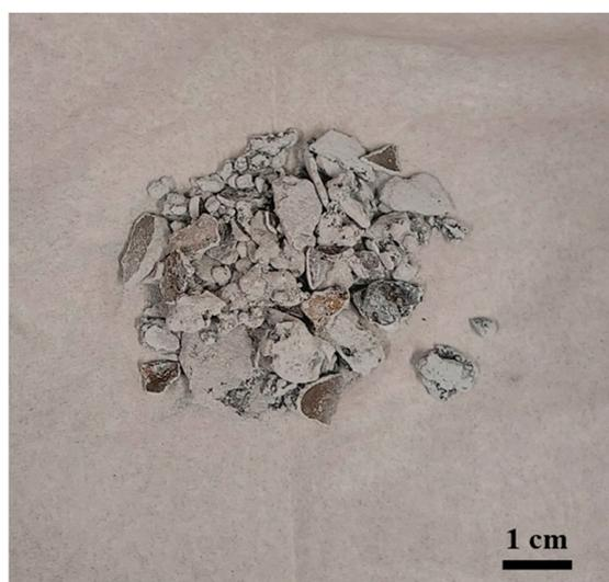
**Figure 8.** The cone part of rutile (TiO<sub>2</sub>) after plasma treatment.
