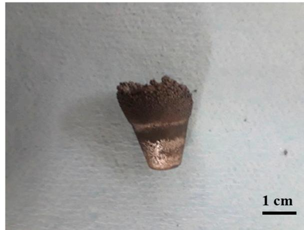
**Figure 12.** The cone part of hematite after plasma treatment.
