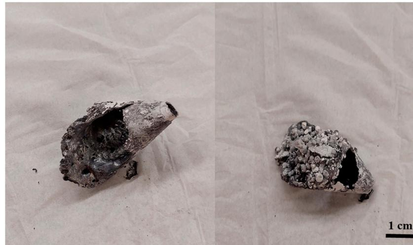
Figure 6. The cone part of alumina after plasma treatment.
