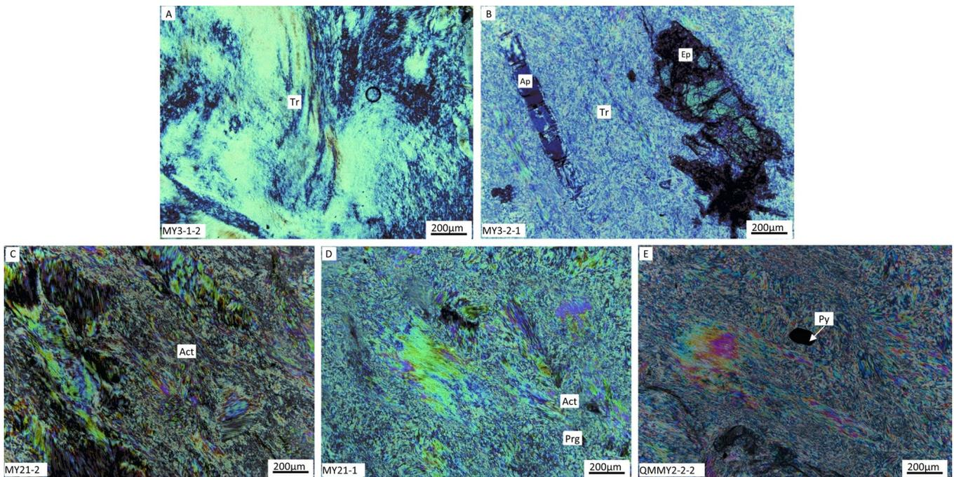
**Figure 6.** Photomicrograph images of Margou nephrite. (A) Different periods of tremolite and brownish dissemination. (B) Two periods of tremolite, TrI and TrII. (C) Distribution of epidote and apatite in fine-grained tremolite aggregates. (D) Irregularly outlined epidote and columnar apatite replaced by tremolite. (E) The opaque metal mineral is pyrite (Tr, tremolite; Act, actinolite; Prg, pargasite; Ep, epidote; Ap, apatite; Py, pyrite).
