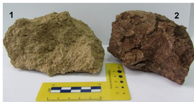
**Figure 2.** Investigated samples from Rujište deposit: 1-light brown clay (sample 1), 2-dark brown-colored clay (sample 2).
