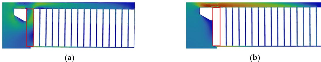
Figure 11. Velocity contours of the air for the effect of insulation between compression plate and laminations: (a) without insulation; (b) with insulation. The red box shows the insulation section.
