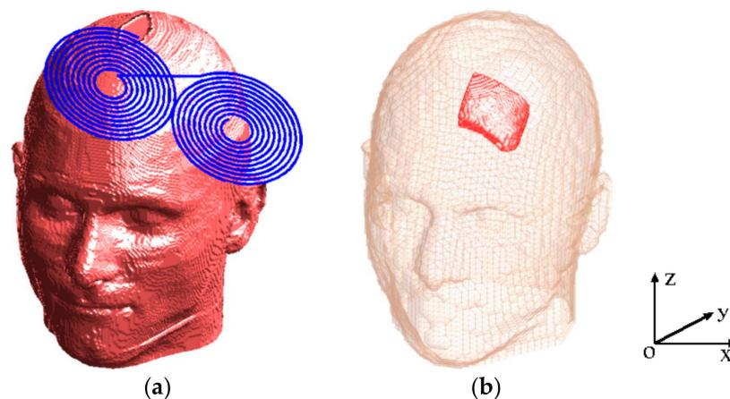
**Figure 1.** The head model with a Fo8 coil (a) and the head model with a titanium skull plate (b).
