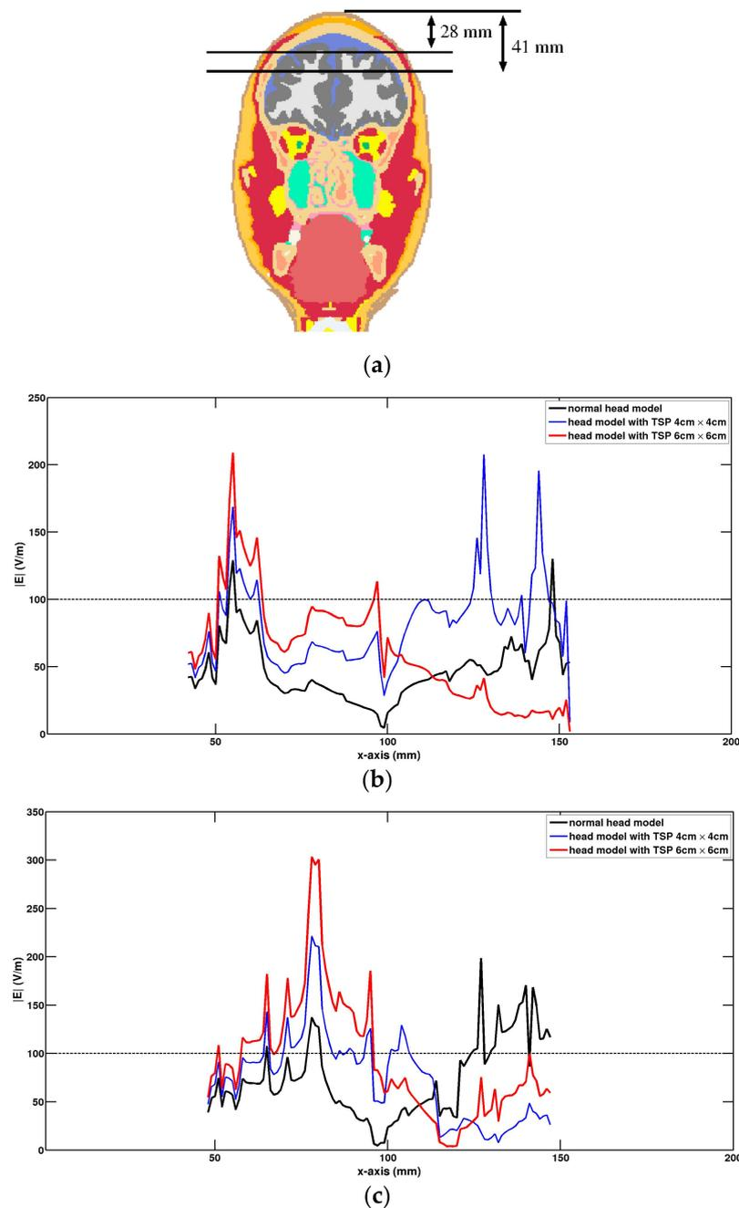
**Figure 6.** Comparison of electric field along the test lines at different depths. (a) Tissue slice at  $y = 80$  mm (coronal plane) with two test lines, (b) test line is situated at a depth of 28 mm, and (c) test line is situated at a depth of 41 mm.
