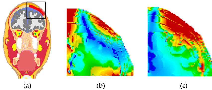
**Figure 3.** Comparison of E-field distribution in head tissues near the TSP. (a) Partially enlarged drawing of tissues, (b) head model with TSP-4cm, and (c) head model without TSP.
