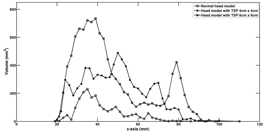
**Figure 5.** Relationship between the brain tissue volume with  $E > 100$  V/m and the field penetration depths.
