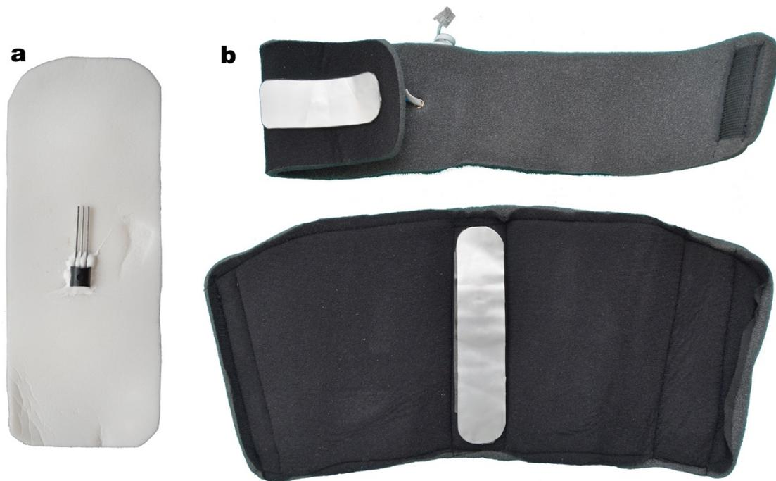
**Figure 4.** (a) Thermal sensor attached to the metallic foil. (b) Thermal sensors for the distal and proximal component.
