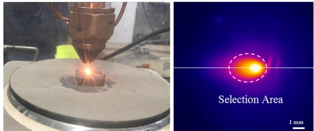
**Figure 3.** Laser-cladding process and infrared image of the laser hot spot on the substrate taken by an IR camera.
