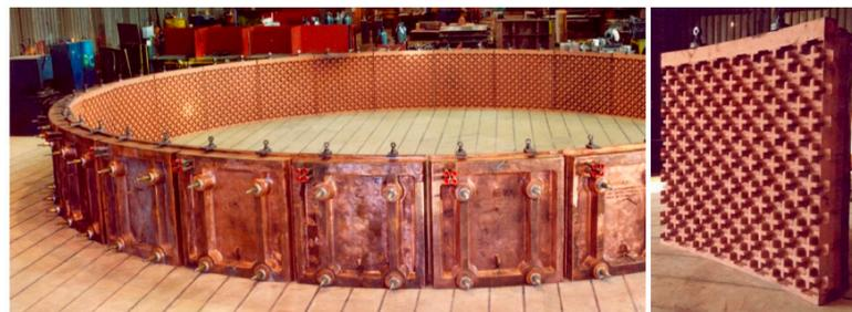
**Figure 13.** An example of Tenova Pyromet’s MAXICOOL® sidewall coolers [31] (reprinted with permission).
