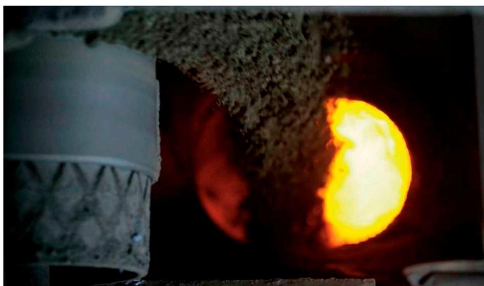
**Figure 10.** Feed input from the top section of the ISASMELT (TSL) [15] (reprinted with permission).
