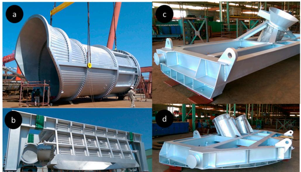
**Figure 11.** AUSMELT TSL (a) Complete furnace shell. (b) Off-gas offtake transition. (c) Furnace roof–upper section with lance port. (d) Furnace roof–lower section with ports for feed and stand-by burner [27] (reprinted with permission).
