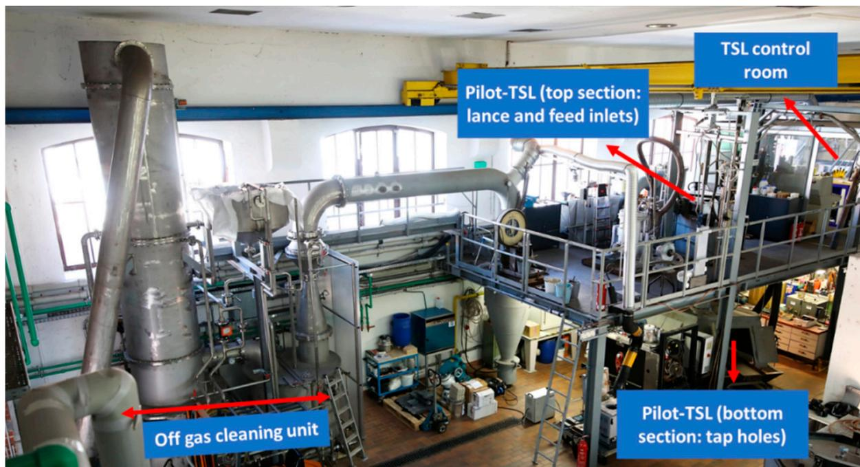
**Figure 9.** Pilot-scale TSL facility at INEMET, TUBAF, Germany [22].
