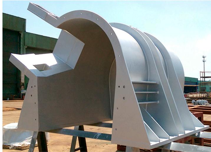
**Figure 4.** The AUSMELT outlet weir for hot products is a separate box bolted to a flanged opening in the furnace shell [11] (reprinted with permission).
