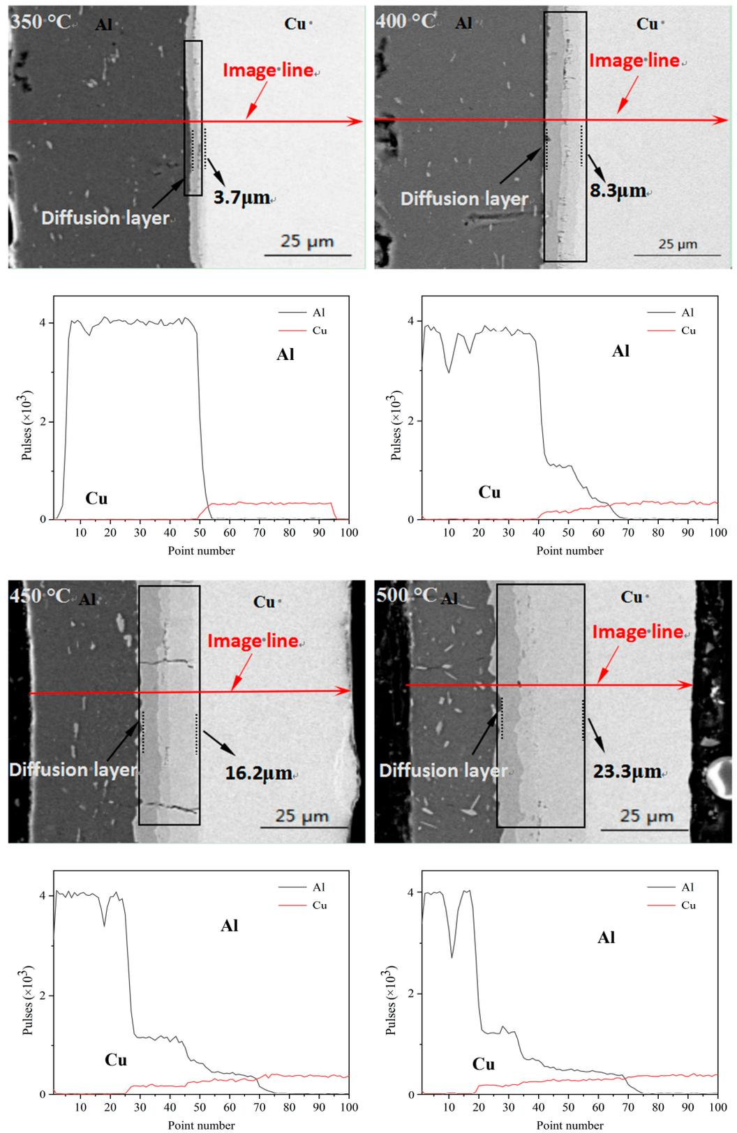
**Figure 4.** Scanning images of interface diffusion layer and element diffusion line of ultra-thin Cu/Al composite sheets at different annealing temperatures.
