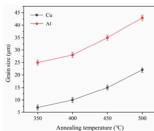
**Figure 3.** Effect of annealing temperature on grain size of ultra-thin Cu/Al composite sheets.
