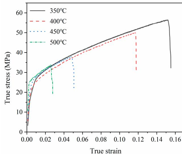
**Figure 7.** True stress–true strain curves of an ultra-thin Cu/Al composite sheet at different annealing temperatures.
