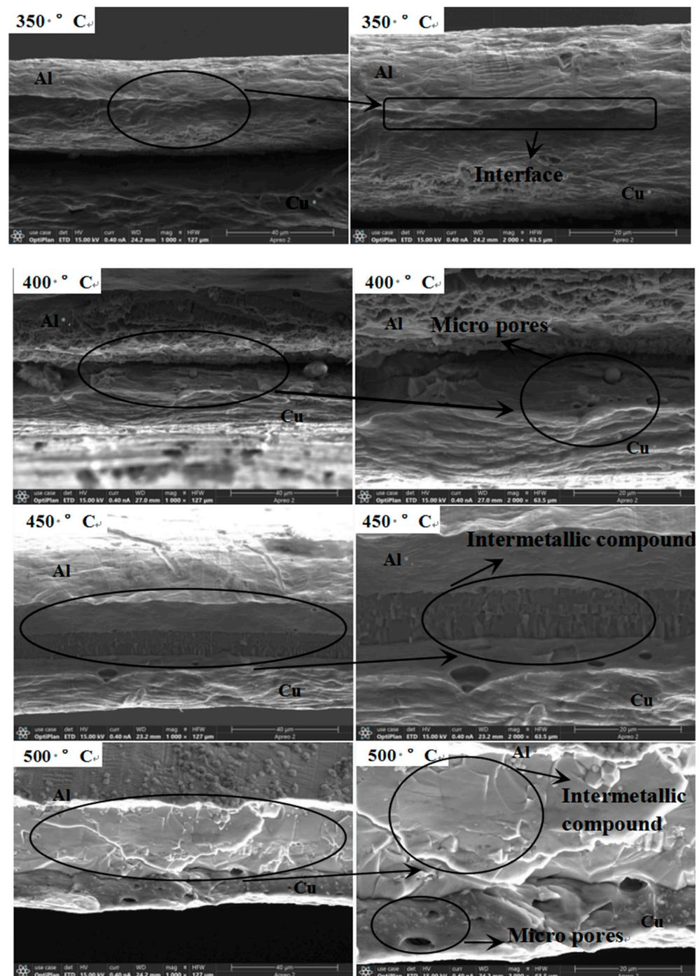
**Figure 8.** Tensile fracture morphology of an ultra-thin Cu/Al composite sheet at different annealing temperatures.
