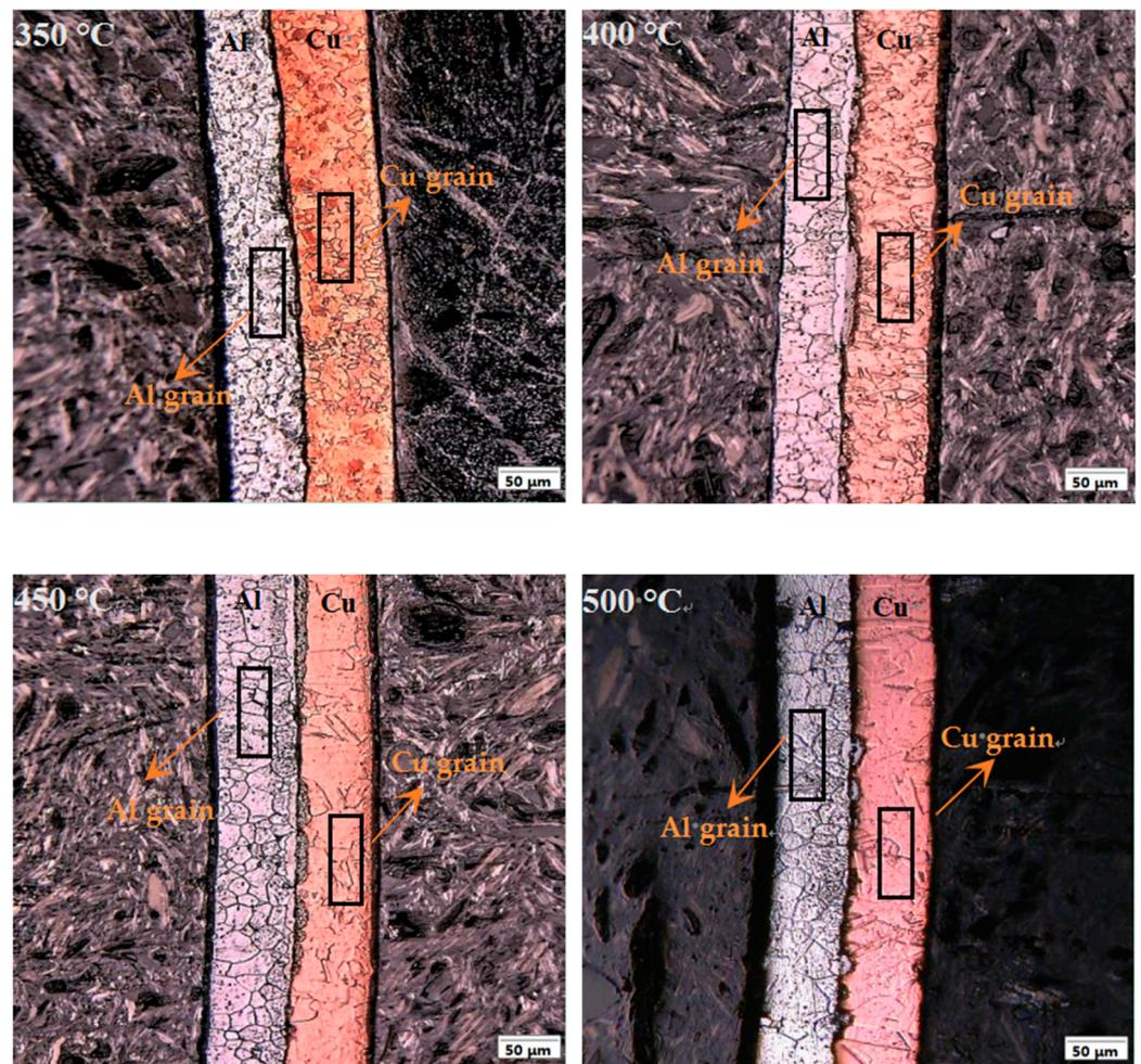
**Figure 2.** Microstructure on the ultra-thin Cu/Al composite sheet interface at different annealing temperatures.
