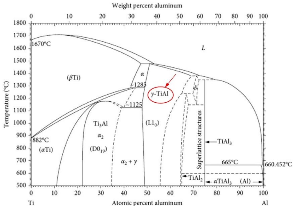
**Figure 1.** Ti-Al binary phase diagram.
