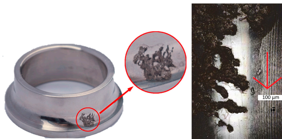
Figure 10. Example for cold-formed bearing damage.
