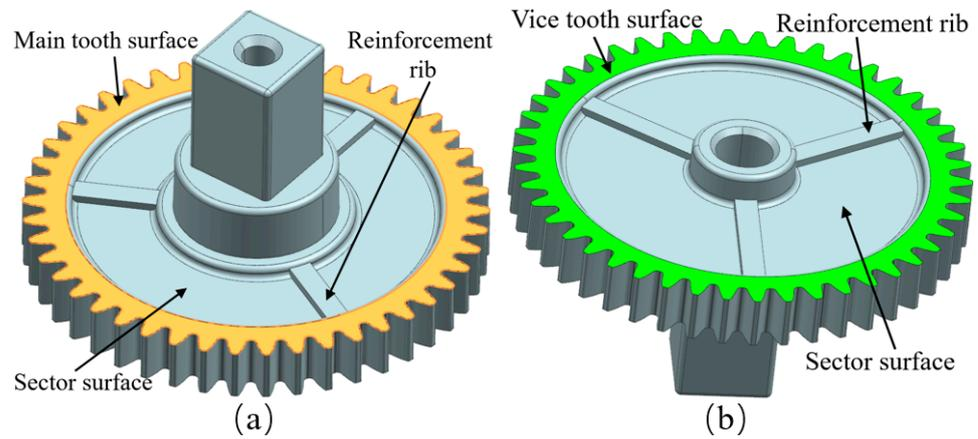
**Figure 11.** Sector surface distribution: (a) Sector surfaces on one side of the main gear surface. (b) Sector surfaces on one side of the vice gear surface.
