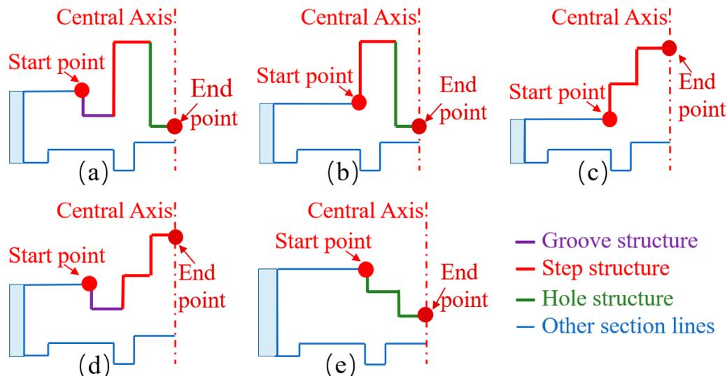
**Figure 6.** The five situations for the interface area: (a) Type 1: groove + step + hole. (b) Type 2: step + hole. (c) Type 3: step. (d) Type 4: groove + step. (e) Type 5: hole.
