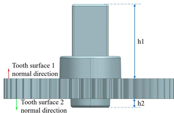
**Figure 10.** Determining the main tooth surface.
