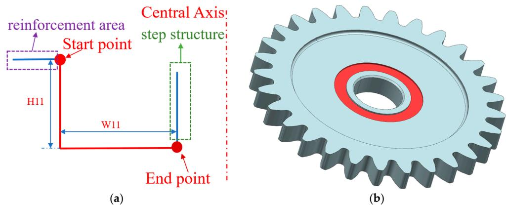
Figure 5. The groove structure: (a) the cross-section line of groove structure and (b) example model.
