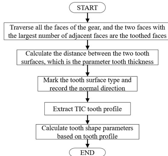
**Figure 8.** Tooth shape parameter calculation process.
