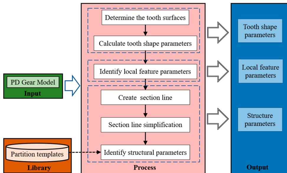
Figure 7. Feature automatic recognition process based on partition templates.
