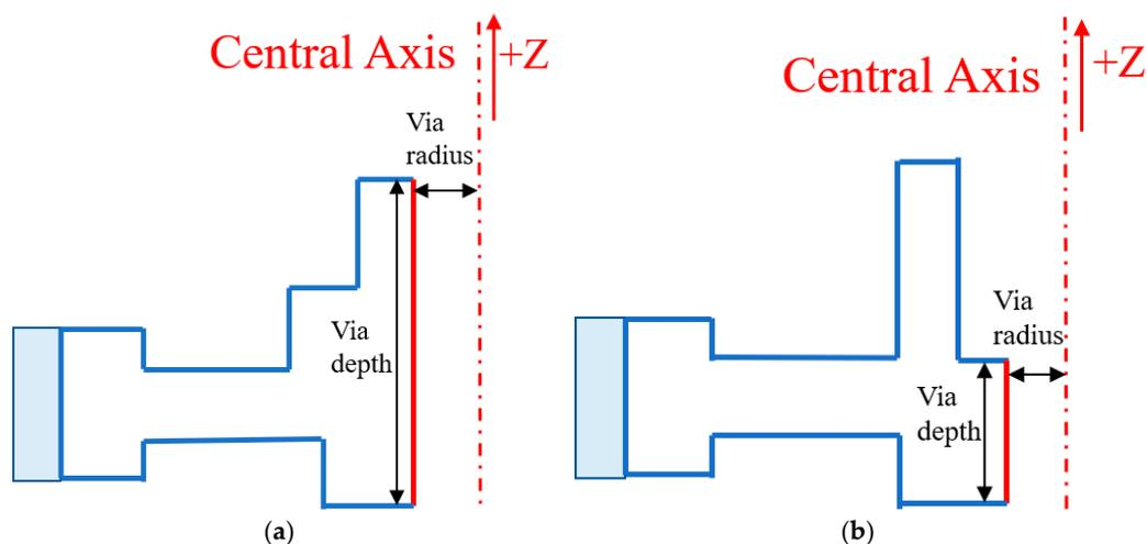
**Figure 4.** The two situations for the via area: (a) through hole and (b) stepped through hole.
