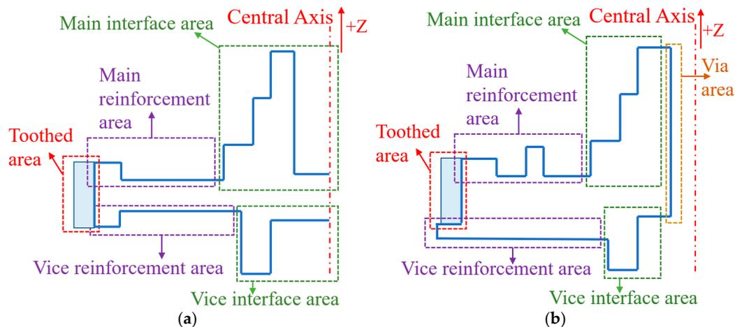
**Figure 3.** The two situations for the cylindrical spur gear feature templates: (a) Both tooth surfaces are TOC. (b) The two tooth surfaces are TOC and TIC, respectively.
