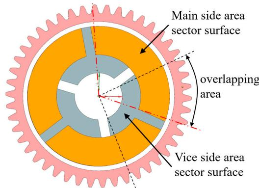
**Figure 12.** Calculation of overlap area of sector surfaces.
