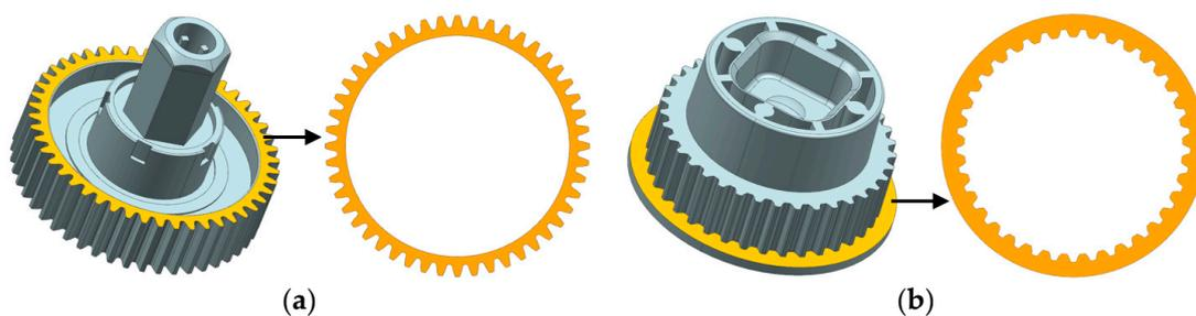
**Figure 2.** The two situations for the gear surface of cylindrical spur gears: (a) The tooth shape is the outer contour. (b) The tooth shape is the inner contour.
