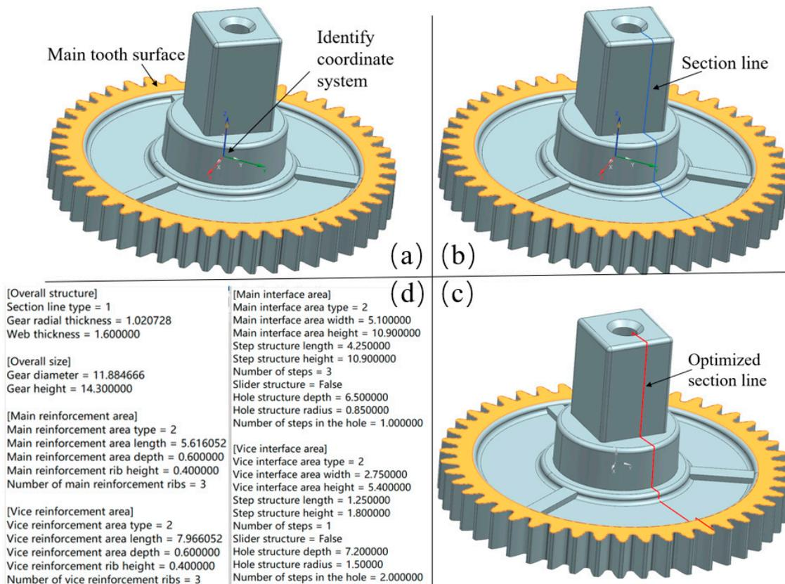
**Figure 9.** Four steps of gear structure parameter recognition: (a) creating identification coordinate system; (b) creating section lines; (c) section line optimization; (d) output structure feature parameters.
