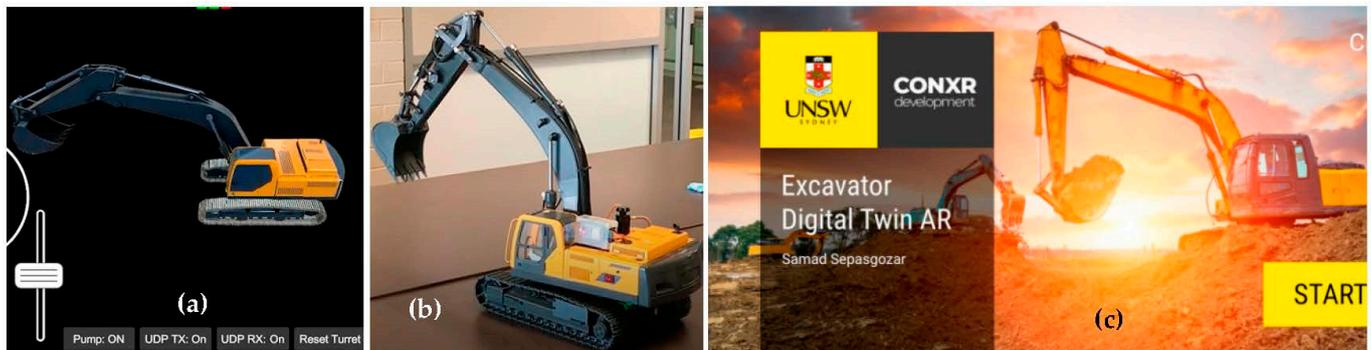
**Figure 9.** Digital and physical objectives in outdoor experimentation. (a) augmented model; (b) physical excavator model; (c) the DT application entrance.
