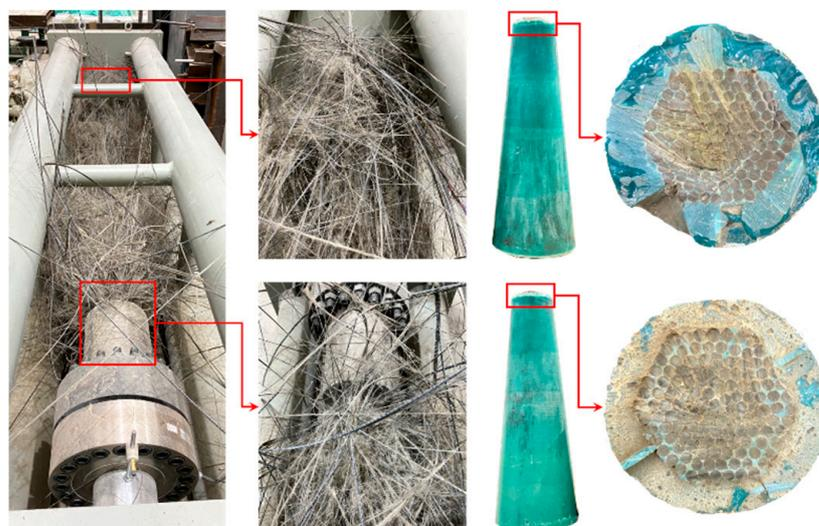
**Figure 12.** Failure mode of the CAS.
