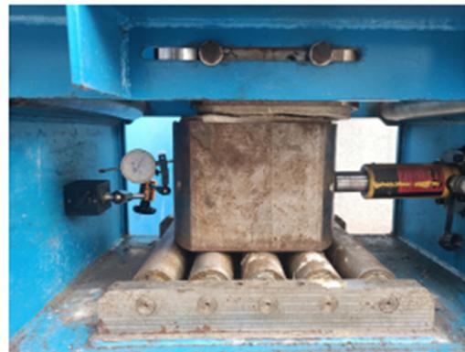
**Figure 2.** Installation of anchorage performance tester and accessories for anchored structural plane.
