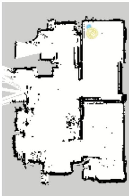
**Figure 12.** 2D Lidar map of site 2: Mock Living Space, location and orientation of the spotlight depicted by the lightbulb symbol.
