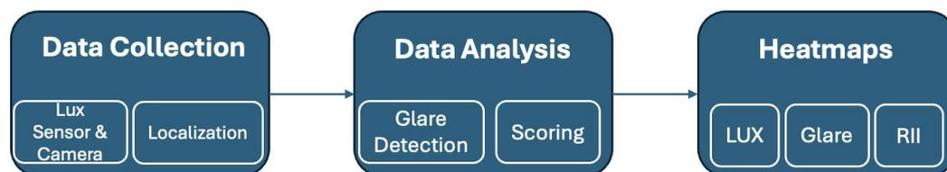
**Figure 1.** Overview of RII-Lux process.
