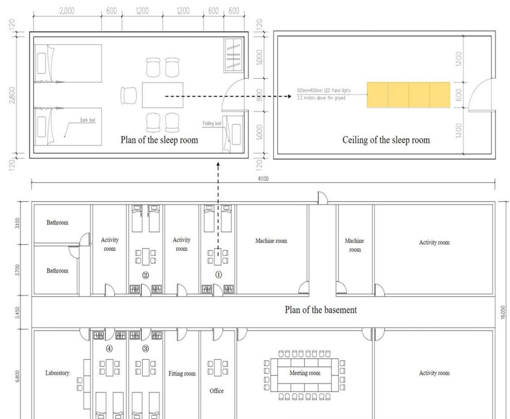
**Figure 1.** Floor plan of the underground laboratory. ①–④ indicated 4 sleep rooms. Each room was equipped with 2 bunk beds, a folding bed, a table and five chairs to accommodate 5 people at a time. The LED panel lights were 2.2 m above the floor directly above the table.
