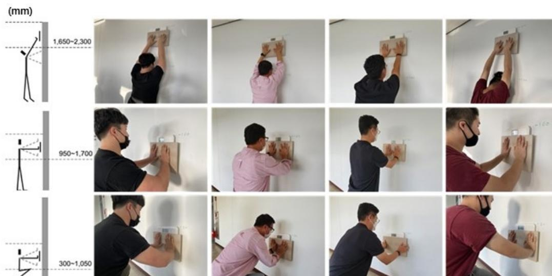
**Figure 3.** Pressurization test for tile pressing according to wall height.
