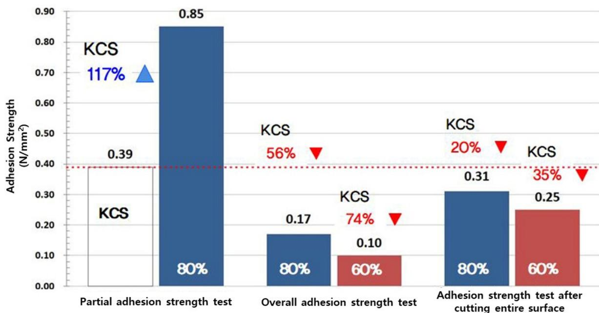
**Figure 13.** Comprehensive comparison table by tile adhesion test results.
