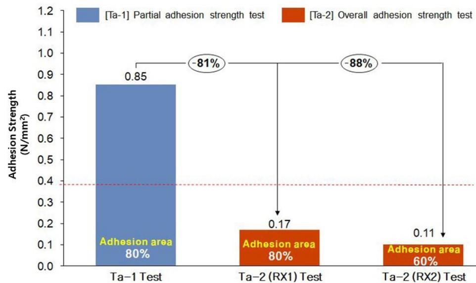
**Figure 8.** Overall adhesion strength test results.
