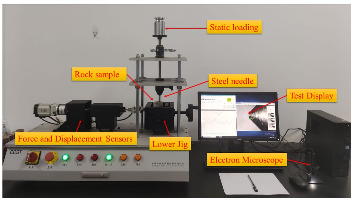
Figure 4. Rock abrasion servo tester.
