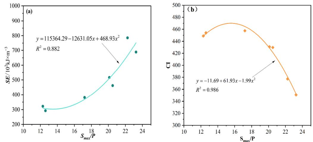
**Figure 8.** Correlations between  $SE$  and  $S_{max}/P$  ratio as well as  $CI$  and  $S_{max}/P$  ratio for hard rock. (a) Correlation between  $S_{max}/P$  ratio and  $SE$ ; (b) correlation between  $S_{max}/P$  ratio and  $CI$ .
