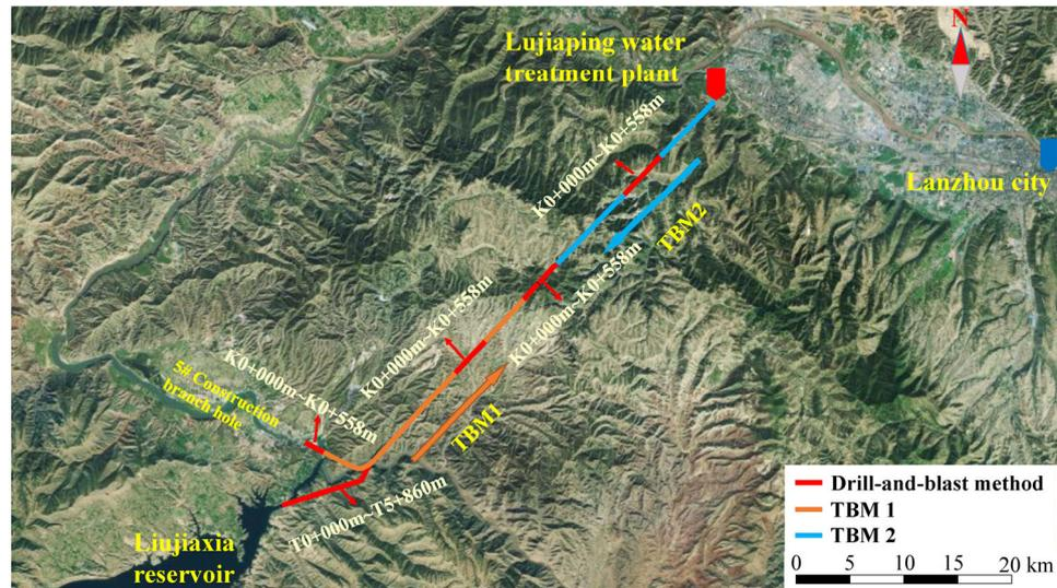
Figure 1. Construction layout of the water conveyance tunnel.
