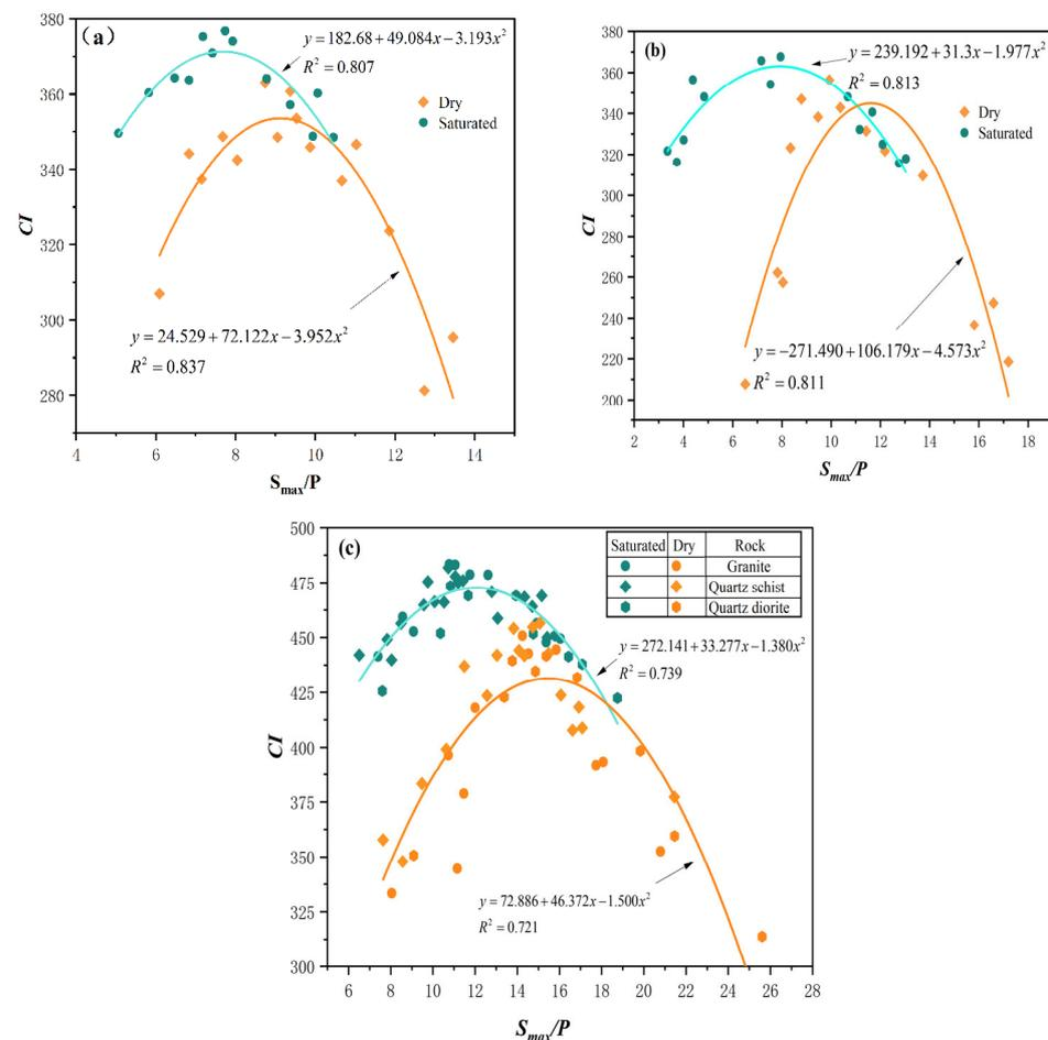
**Figure 10.**  $CI$  and  $S_{max}/P$  ratio relationship curves in dry and saturated conditions. (a) Relatively soft rock, (b) medium-hard rock, and (c) hard rock.
