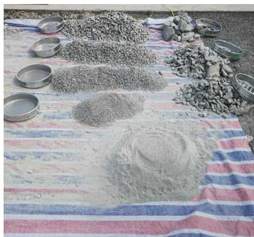
**Figure 3.** The sieving test of TBM rock chips.
