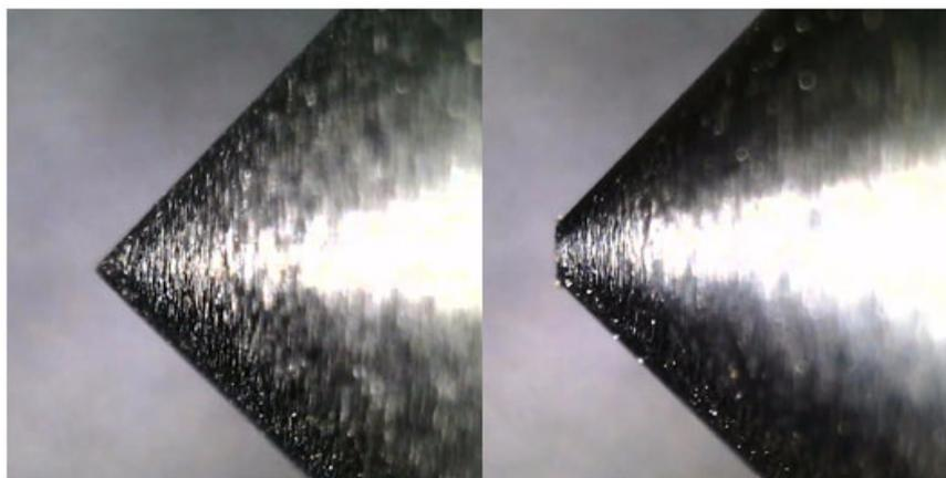
Figure 5. Steel needle evaluation before and after the Cerchar abrasion test.
