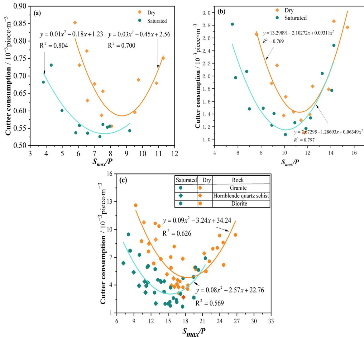
**Figure 12.** Cutter consumption variation with  $S_{max}/P$  ratio in dry and saturated conditions. (a) Relatively soft rock, (b) medium-hard rock, and (c) hard rock.
