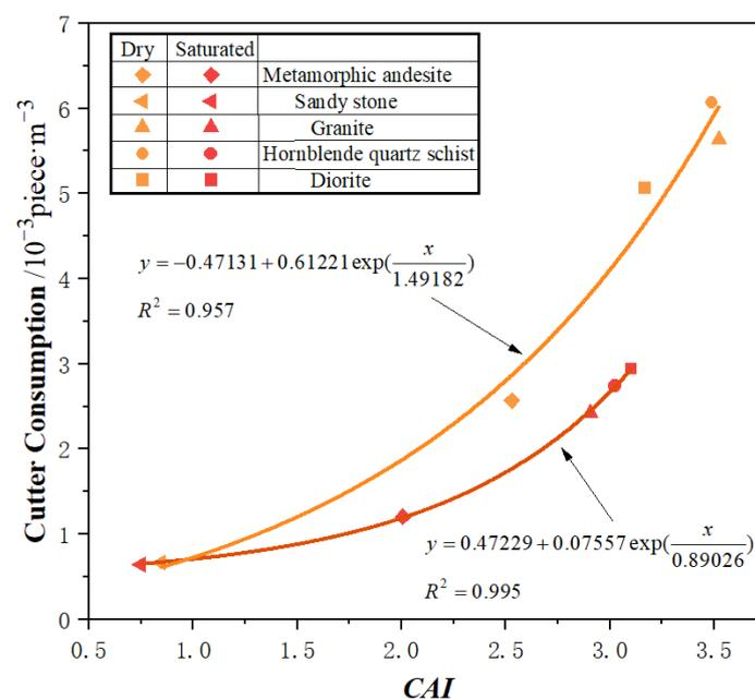
**Figure 11.** Cutter consumption variation with  $CAI$  in dry and saturated conditions.
