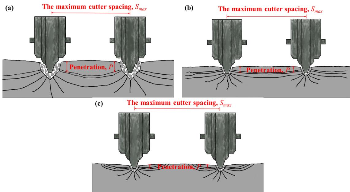
**Figure 9.** Disc cutter rock-breaking methods at different  $S_{max}/P$  values. (a) Smaller  $S_{max}/P$  value, (b) optimal  $S_{max}/P$  value, and (c) greater  $S_{max}/P$  value.
