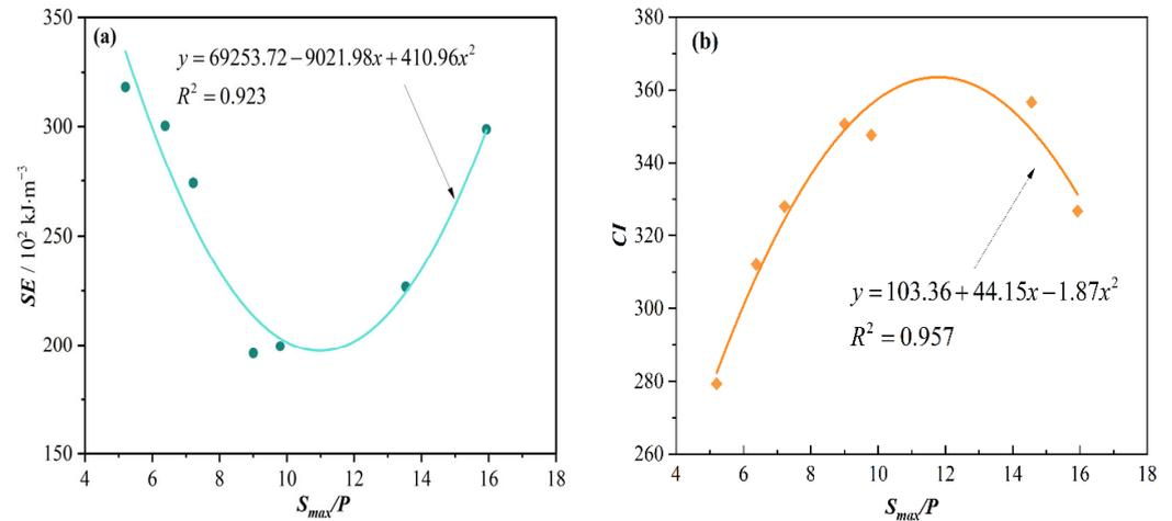
**Figure 7.** Correlations between  $SE$  and  $S_{max}/P$  ratio and  $CI$  and  $S_{max}/P$  ratio for soft rock. (a) Correlation between  $S_{max}/P$  ratio and  $SE$ ; (b) correlation between  $S_{max}/P$  ratio and  $CI$ .
