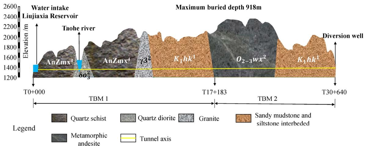
Figure 2. Geological profile of the water conveyance tunnel.
