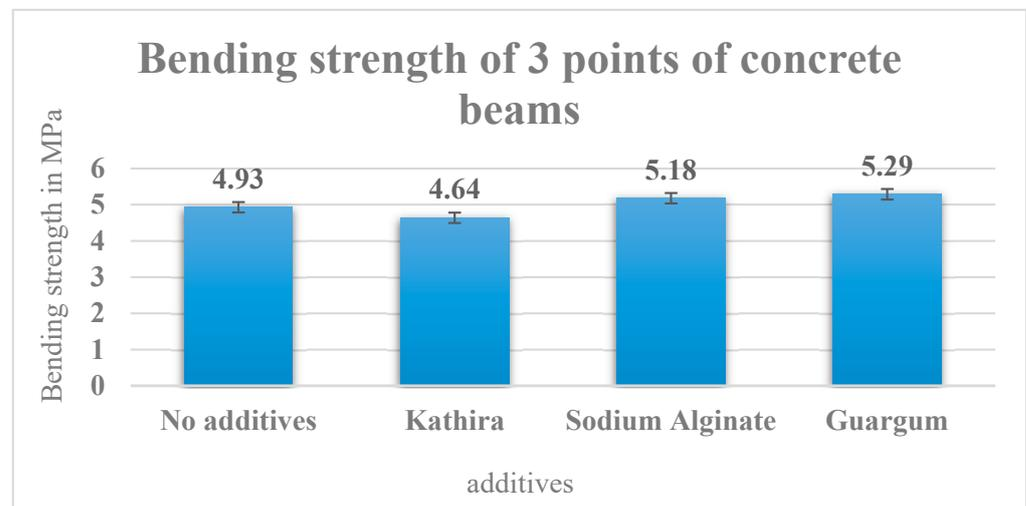
**Figure 23.** 3-point bending strength test results of concrete beam.
