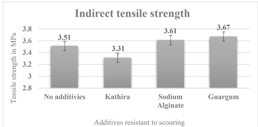
**Figure 22.** Indirect tensile strength test results.
