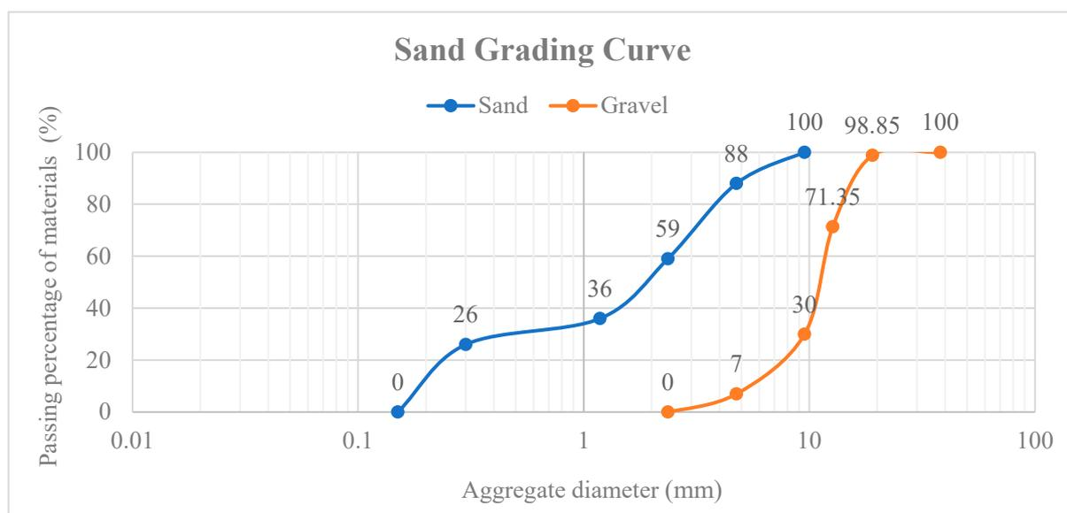
**Figure 1.** Sand grading curve.
