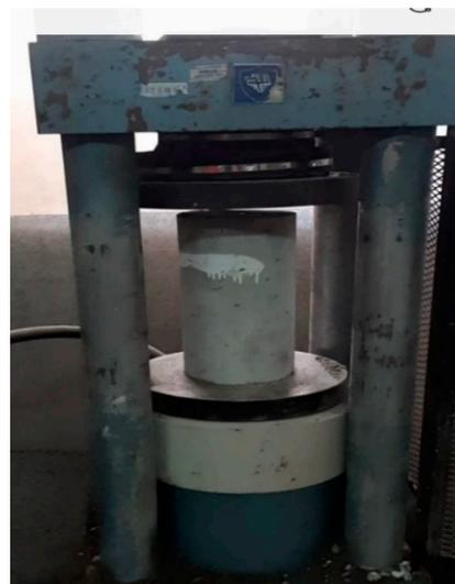
**Figure 11.** Compressive strength measuring device.
