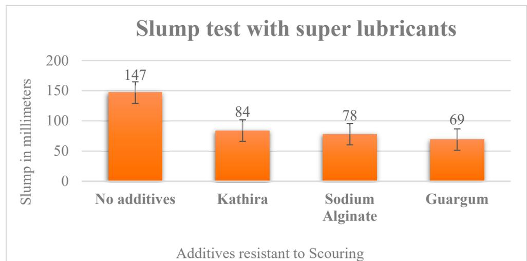
**Figure 17.** Slump test results using super lubricants.
