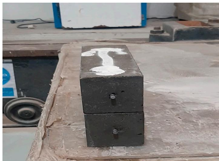
**Figure 15.** Specimens made for shrinkage testing.
