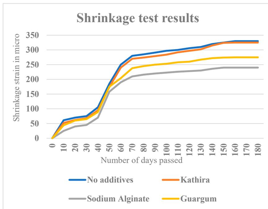
**Figure 24.** A graph of the results of the shrinkage test.
