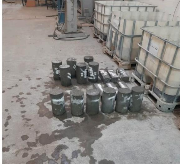
**Figure 10.** Samples removed from water ponds saturated with lime.
