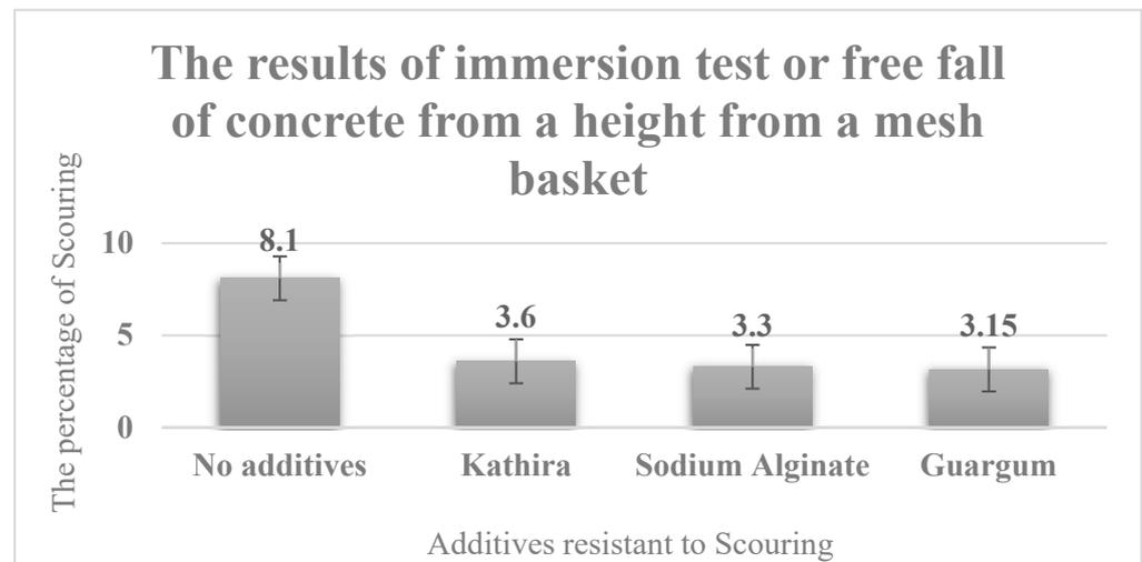
**Figure 18.** The results of concrete immersion or free fall test from mesh basket.
