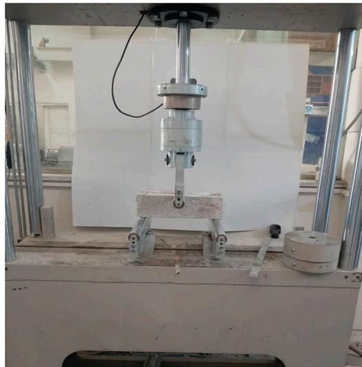
**Figure 14.** The 3-point bending strength test of the concrete beam.
