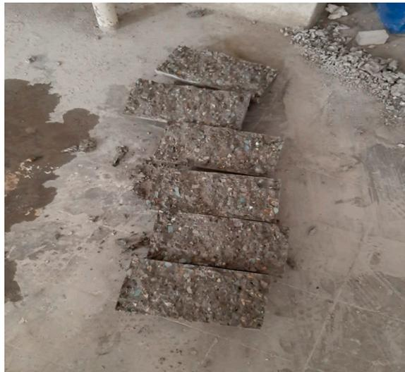
**Figure 13.** A number of broken concrete samples in indirect tensile test.
