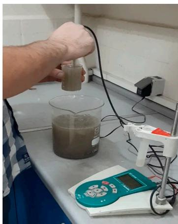
**Figure 8.** Measuring the dissolution rate of concrete cement with a PH meter.
