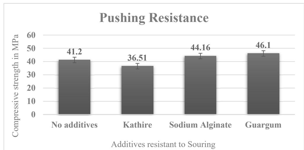
**Figure 21.** Graph of compressive strength test results.
