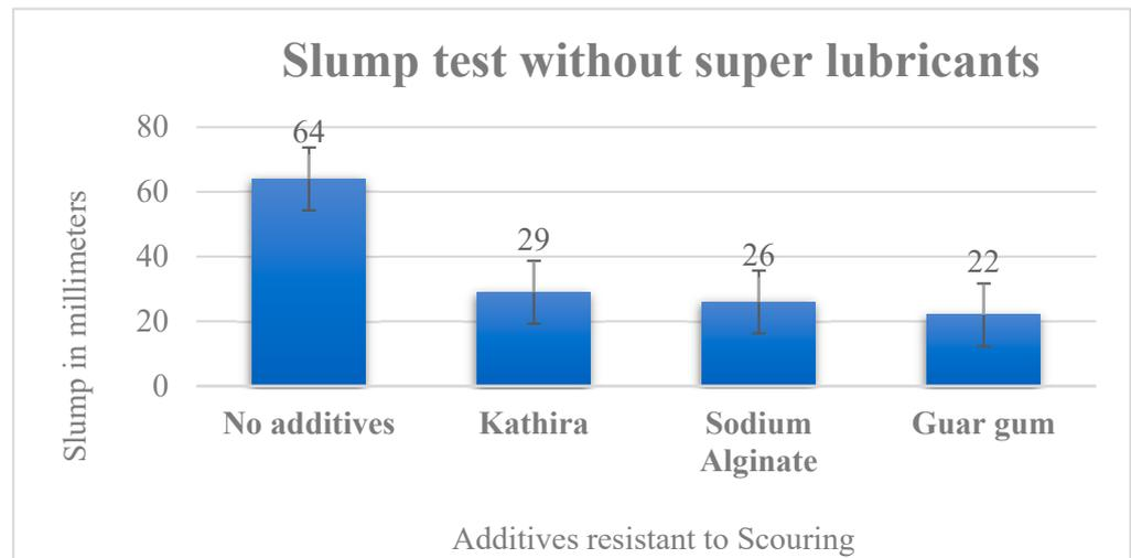
**Figure 16.** Slump test results without using super lubricants.
