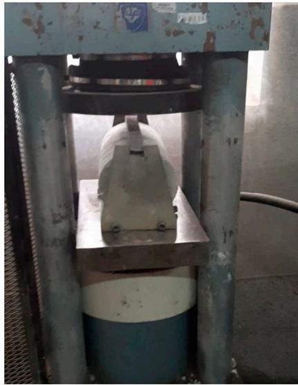
**Figure 12.** Cylindrical concrete specimen inside a steel sheath for indirect tensile test.
