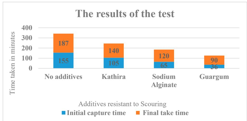
**Figure 20.** Results of setting time test of fresh concrete.
