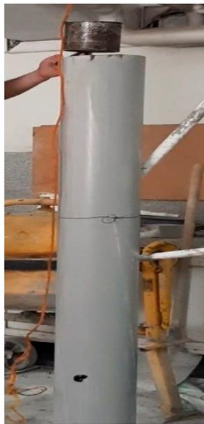
**Figure 7.** Fresh concrete scouring test device.
