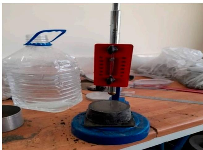
**Figure 9.** Vicat device for measuring concrete setting time.
