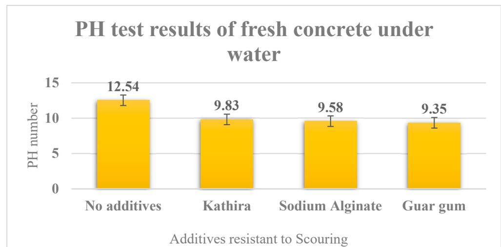
**Figure 19.** PH test results of fresh concrete under water.
