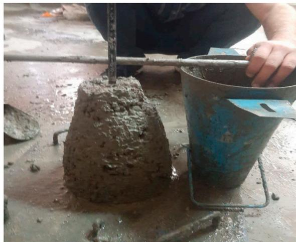
**Figure 6.** Measurement of concrete slump.
