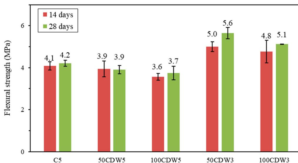
Figure 9. Flexural strength of concrete.
