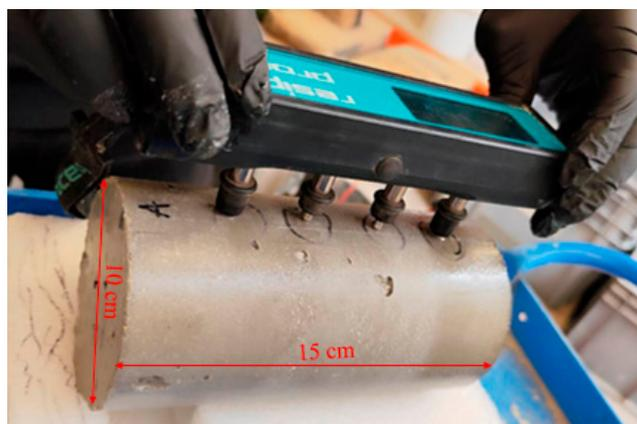
**Figure 3.** Electrical resistivity test.
