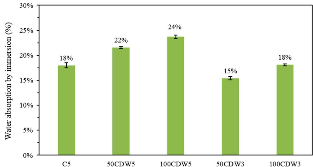
**Figure 7.** Water absorption by immersing the concrete.
