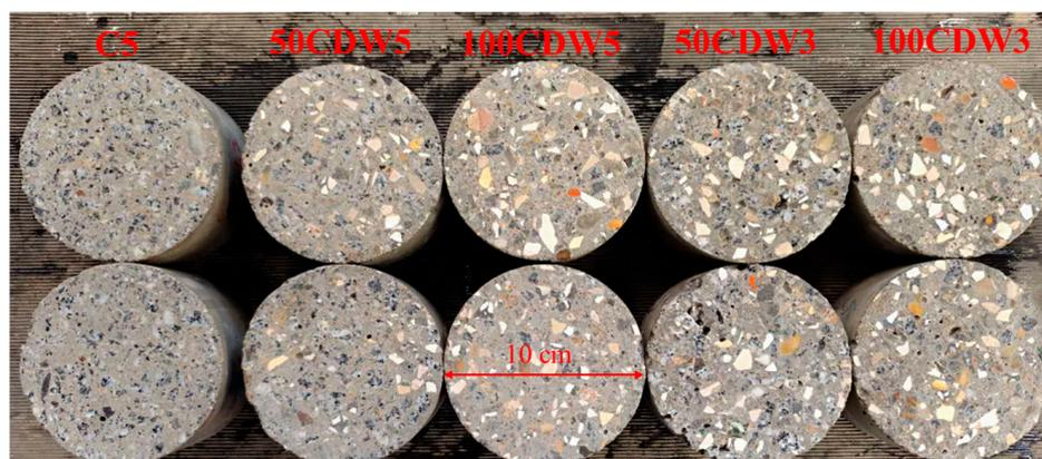
**Figure 4.** Specimen preparation for the chloride penetration test.
