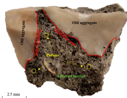
**Figure 1.** A particle of the recycled concrete aggregate used.
