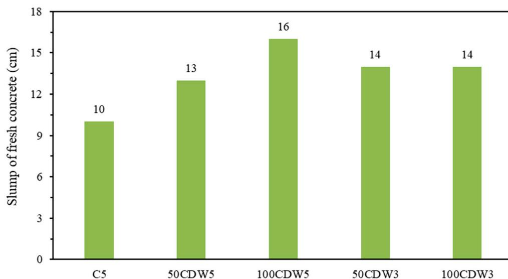
**Figure 5.** Slumps of fresh concrete.
