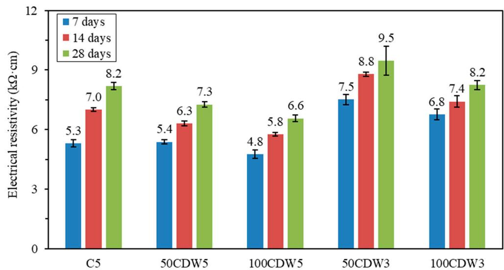
Figure 10. Electrical resistivity of concrete.
