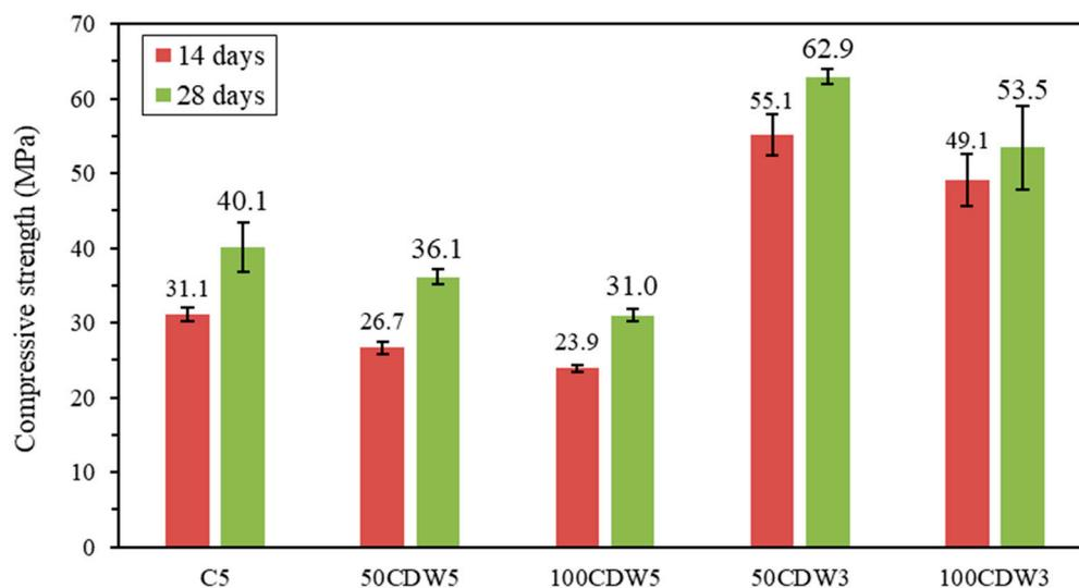
**Figure 8.** Compressive strength of concrete.
