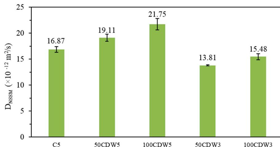
**Figure 11.** Non-steady-state migration coefficient of concrete.
