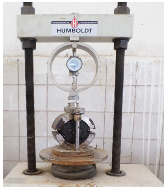
**Figure 4.** Marshall test (HUMBOLDT).
