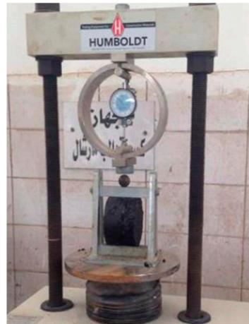
**Figure 7.** Instrument for indirect tensile test.
