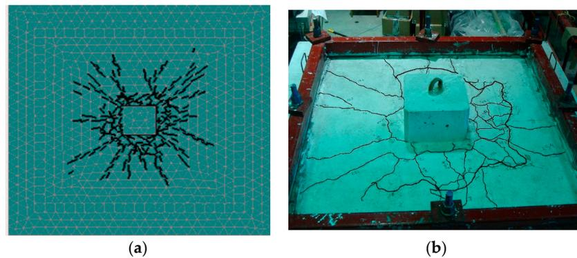
**Figure 5.** Cracks' schematic (tension side). (a) FE slab; (b) Experimental [3].
