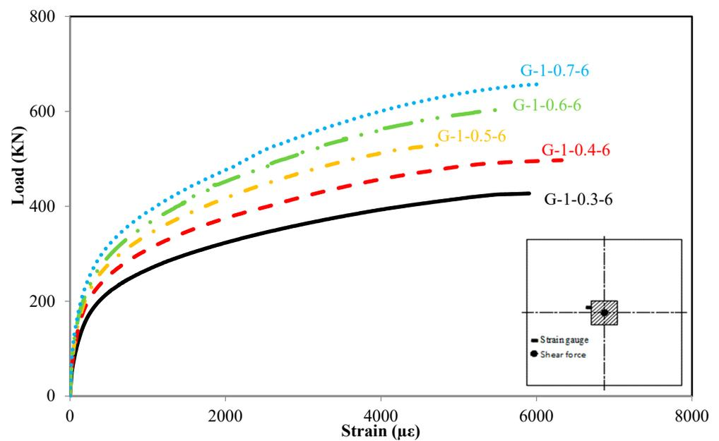
(b) Slabs with different perimeter-to-depth ratios
