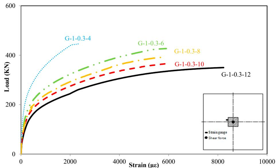
(c) Slabs with different span-to-depth ratios
