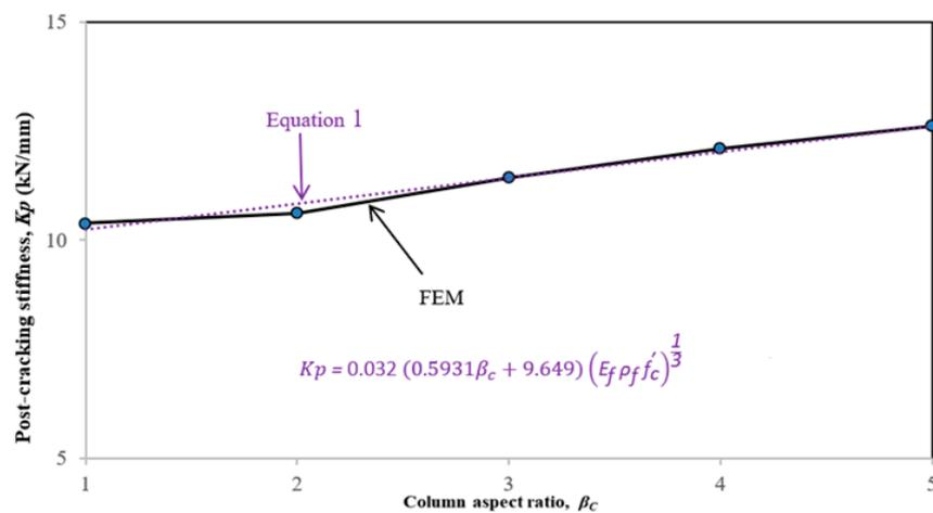
Figure 9. Post-cracking stiffness versus column–aspect ratio.
