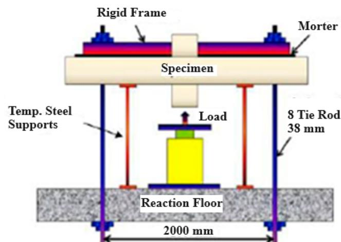
Figure 2. Three-dimensional test setup.
