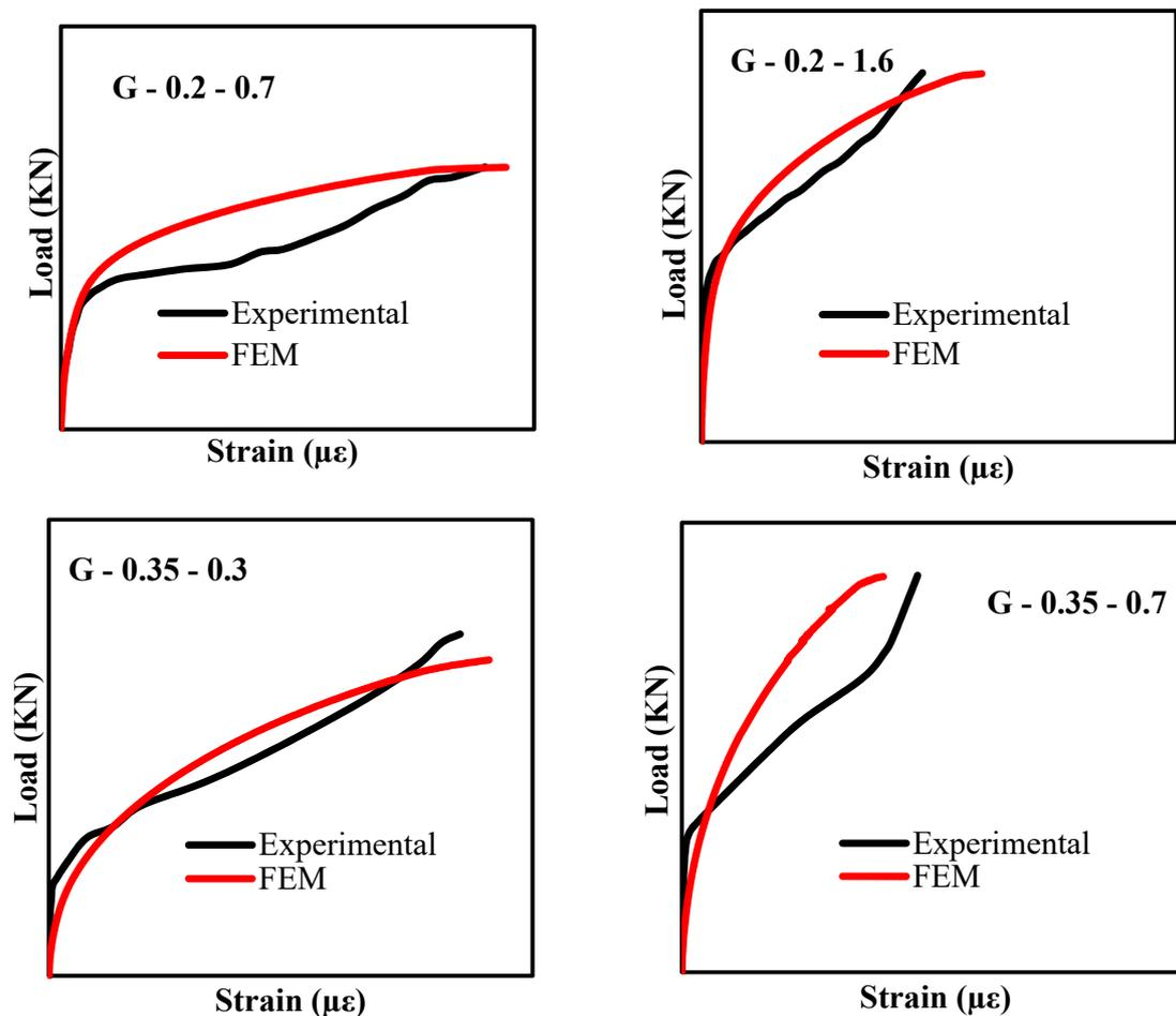
**Figure 7.** Load–reinforcement strains at the column face.
