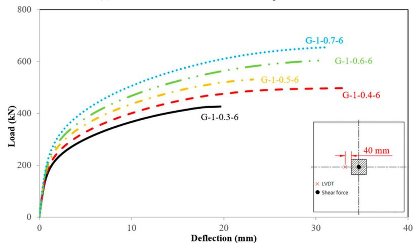
(b) Slabs with different perimeter-to-depth ratios
