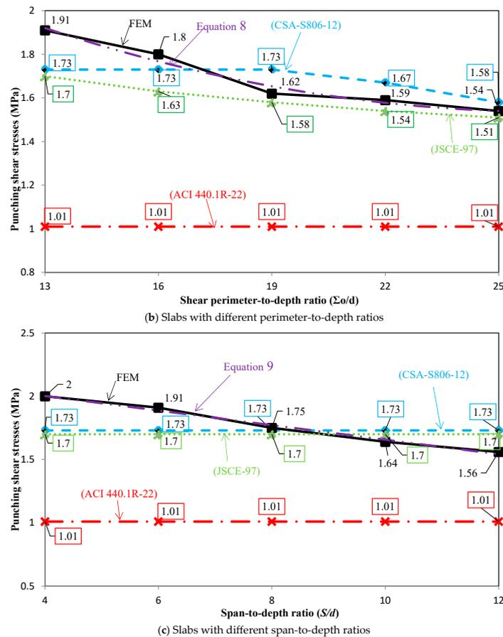
Figure 11. Punching shear stresses.
