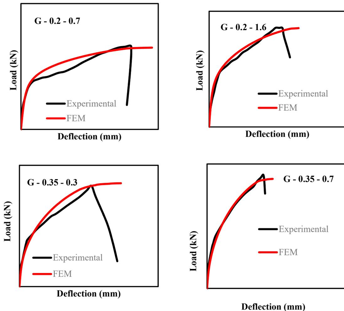
**Figure 6.** Load–deflection at 40 mm from the column face.
