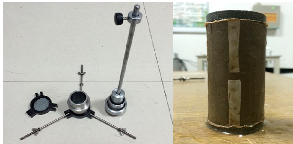
Figure 2. Triaxial reconstituted soil specimen preparation apparatus and soil sample [5].
