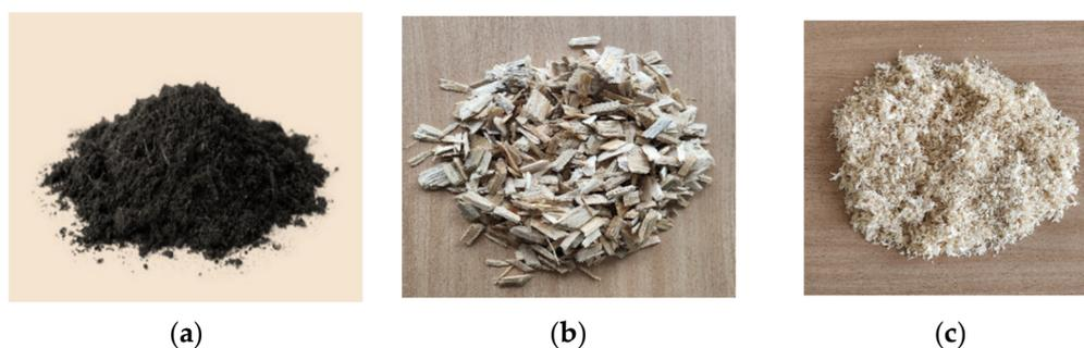
**Figure 2.** Filter materials used in the experiments: (a) peat; (b) wood chips; and (c) sawdust.
