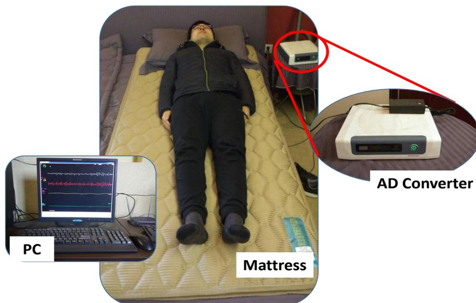
**Figure 2.** The micro-movement sensitive mattress-based BCG signal acquisition system (RS-611).
