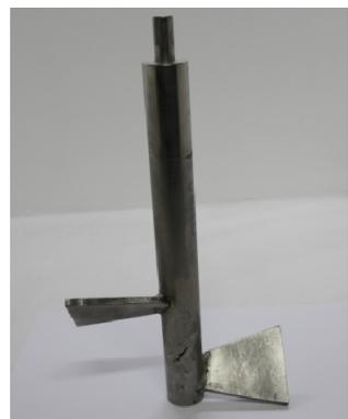
**Figure 2.** Polygonal Impeller B.
