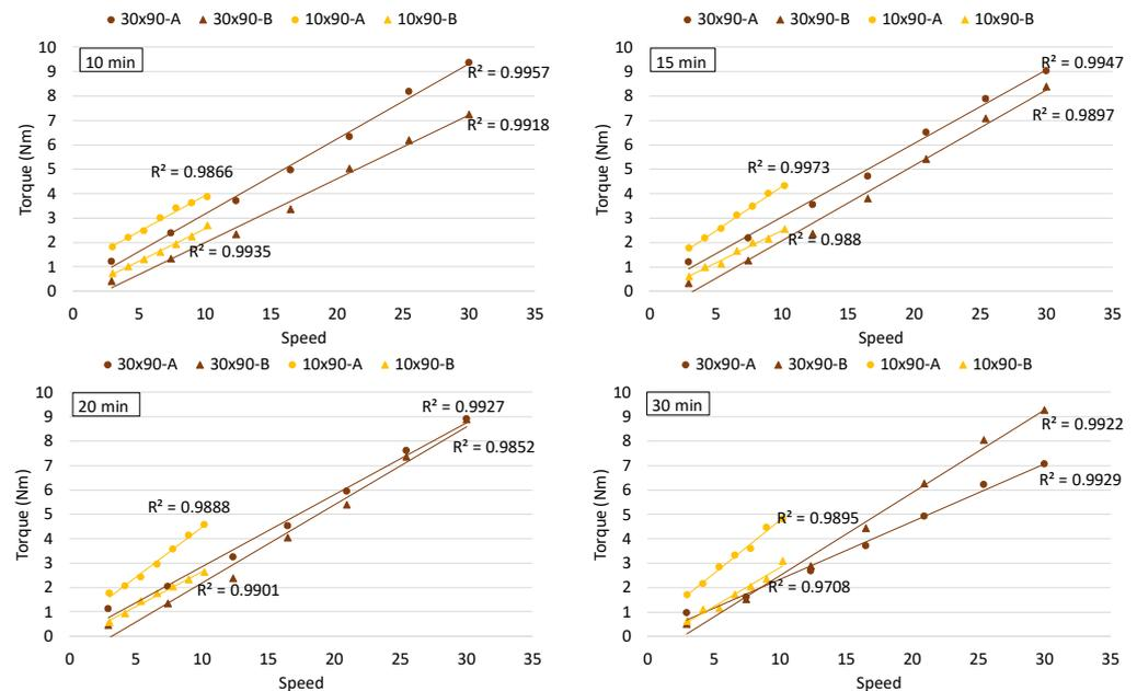
Figure 13. Flow curves of the mixes.
