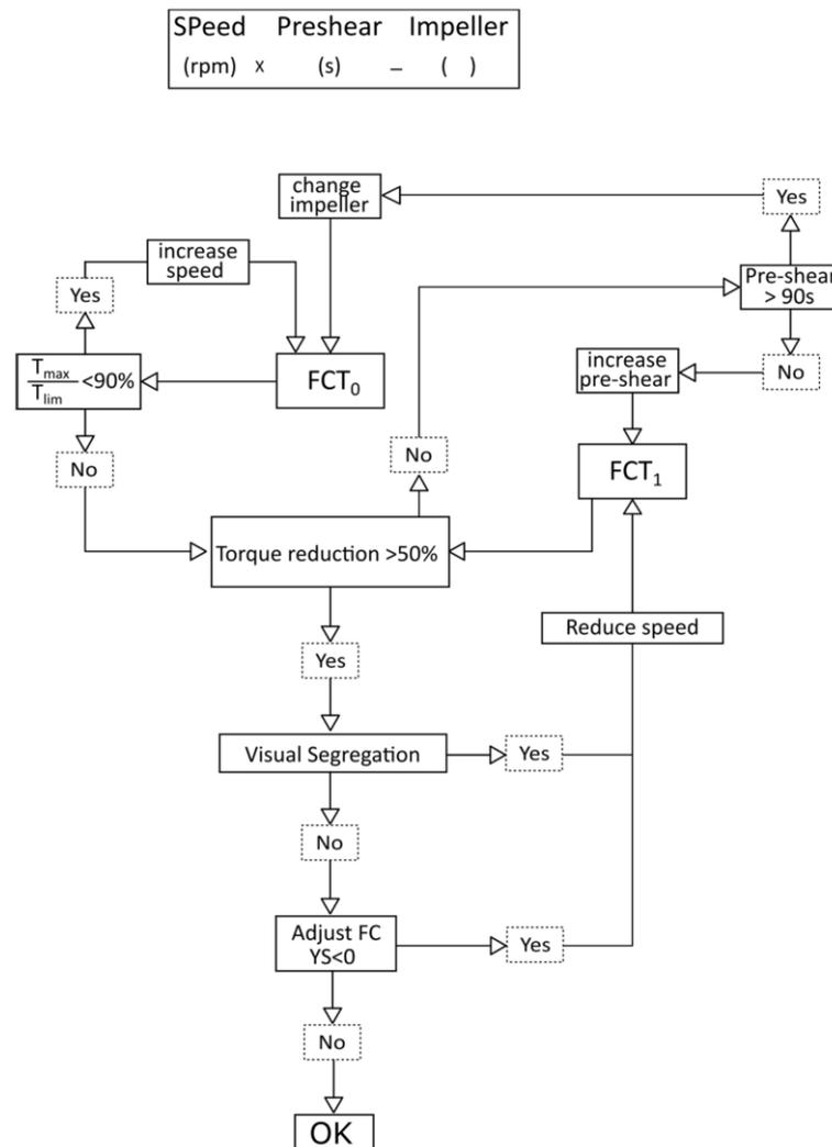
Figure 18. Adjustment flow chart.
