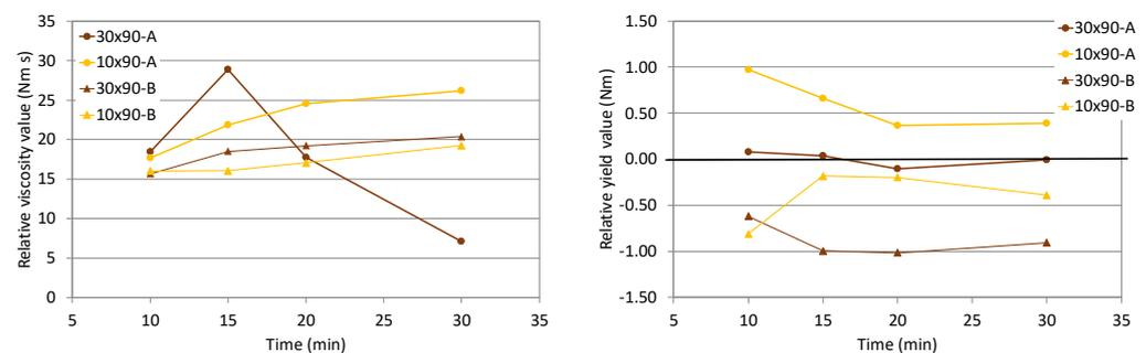
Figure 14. Relative yield stress and relative plastic viscosity.
