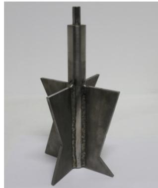
**Figure 1.** Polygonal Impeller A.
