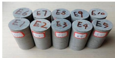
Figure 1. Limestone specimens.
