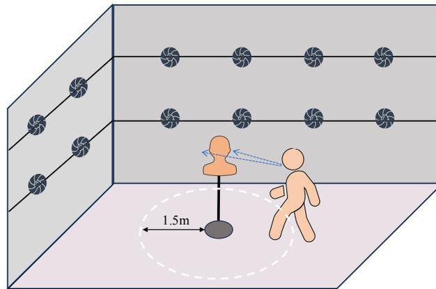
**Figure 4.** Side view of capture layout. The speaker speech is recorded with a head-mounted microphone and the binaural audio is captured with binaural microphones on the ears of the mannequin. Mannequin and participant positions are tracked with OptiTrack cameras mounted on the walls of the room.
