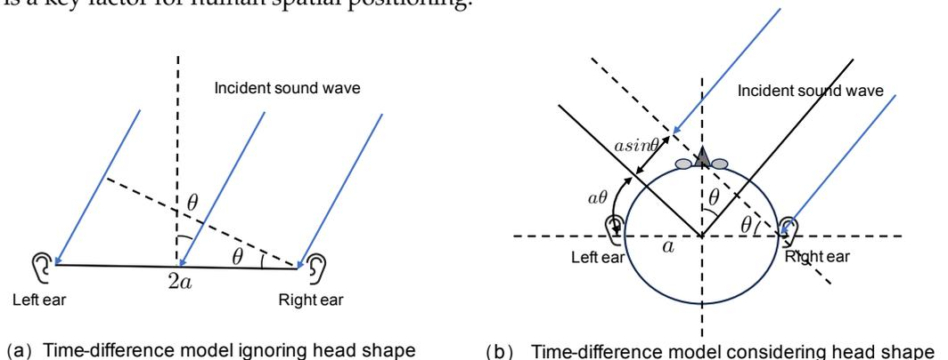
**Figure 3.** Schematic diagram of horizontal ITD (interaural time difference) calculation.
