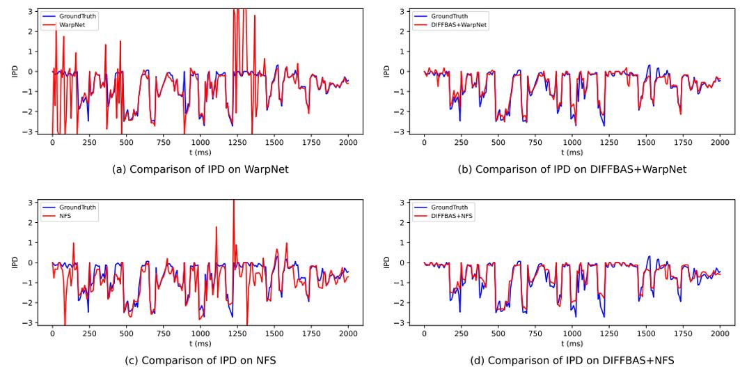
**Figure 6.** Comparison of IPD(interaural phase difference) at frequencies with peak energy over a two-second period compared to recording audio. The range of IPD is  $[-\pi, \pi]$ . The blue line represents the changing trend of recording audio, and the red line represents the changing trend of binaural audio synthesized by the model.
