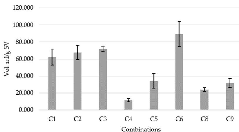
**Figure 1.** Biogas production obtained for each evaluated combination.
