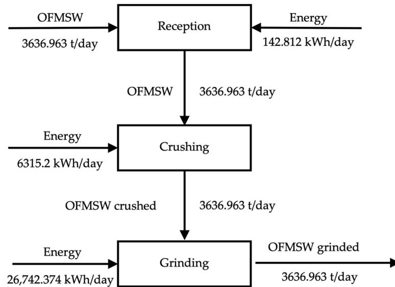
Figure 4. Substrate preparation stage.
