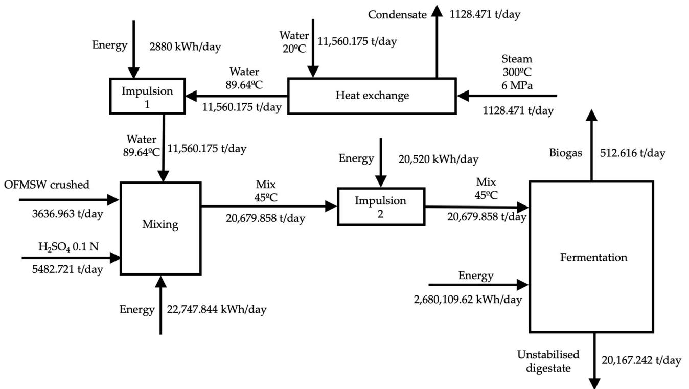
Figure 5. Mixing and fermentation stage.
