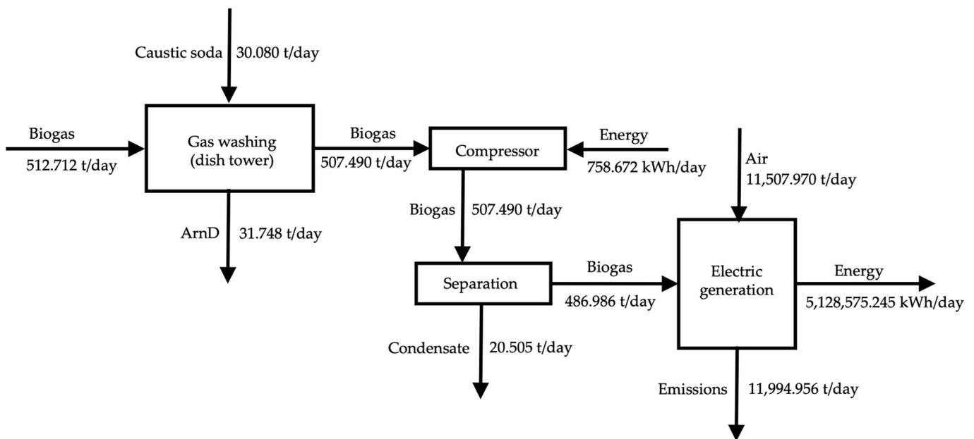
**Figure 6.** Biogas purification and power generation stage.
