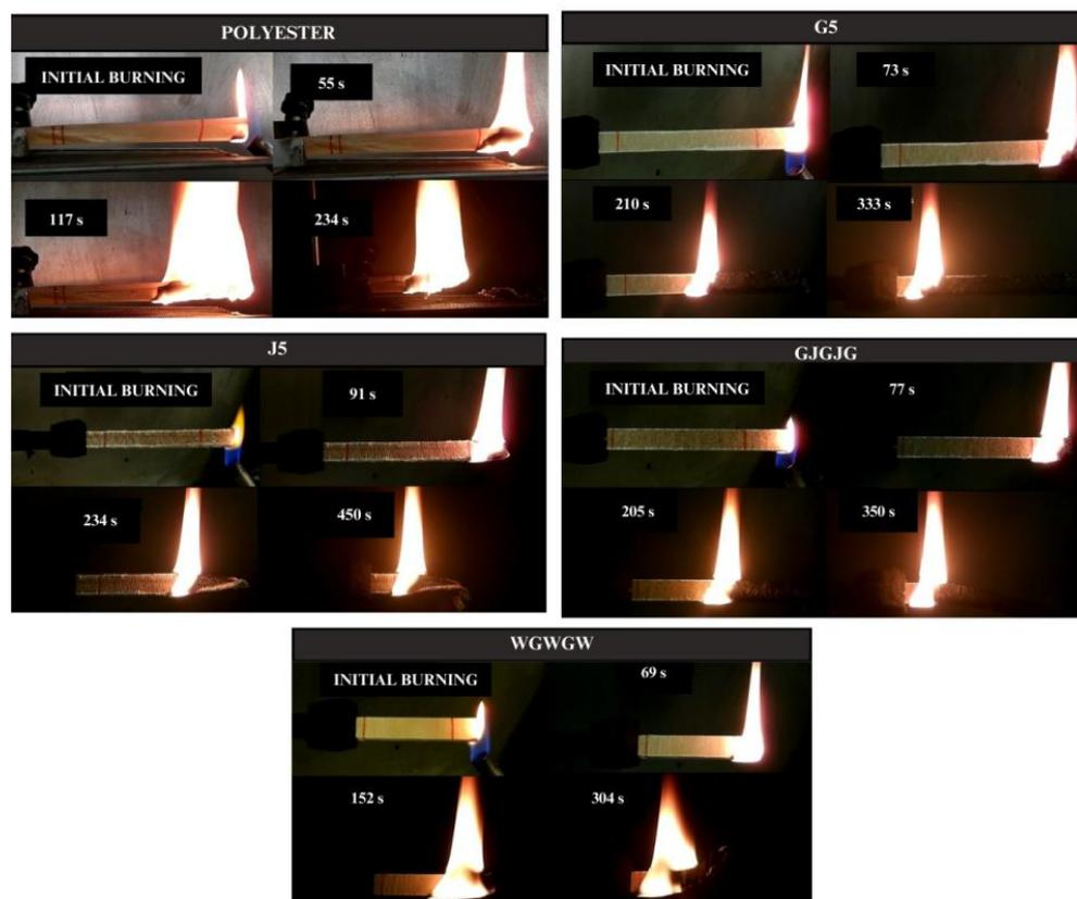
**Figure 8.** Appearance of the samples during the horizontal firing test in accordance with UL 94.
