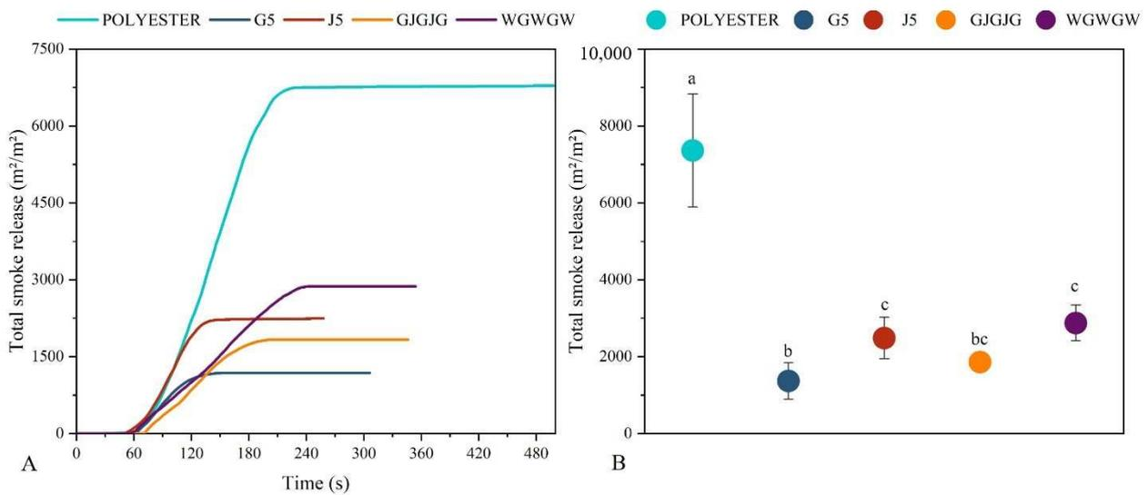
**Figure 5.** Total smoke release as a function of time for each group analyzed (A) and average values for total smoke release at the end of the test (B). Different letters above the errors in each group represent a statistical difference.
