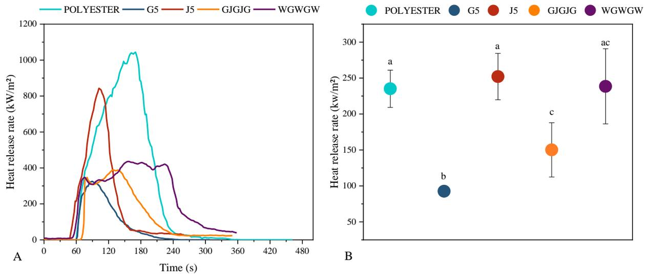
**Figure 2.** Heat release rate as a function of time for each group analyzed (A) and the average values of the heat release rate and confidence interval of 95% (B). Different letters above the errors in each group represent a statistical difference.
