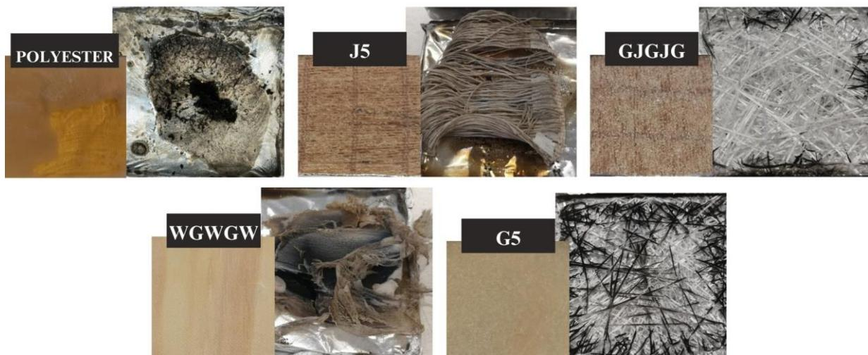
**Figure 3.** Appearance of the samples before and after the cone calorimeter tests.
