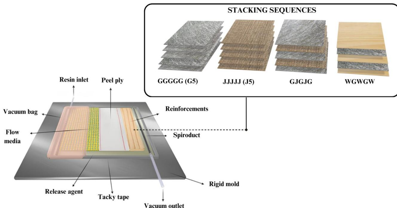
**Figure 1.** Representation of the VIP for manufacturing the laminates and their different stacking sequences.
