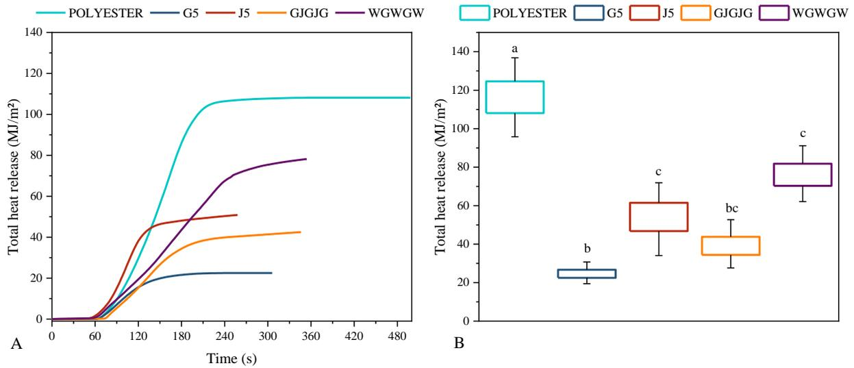
**Figure 4.** Total heat release (THR) as a function of time for each group analyzed (A) and average maximum values for THR (B). Different letters above the errors in each group represent a statistical difference.
