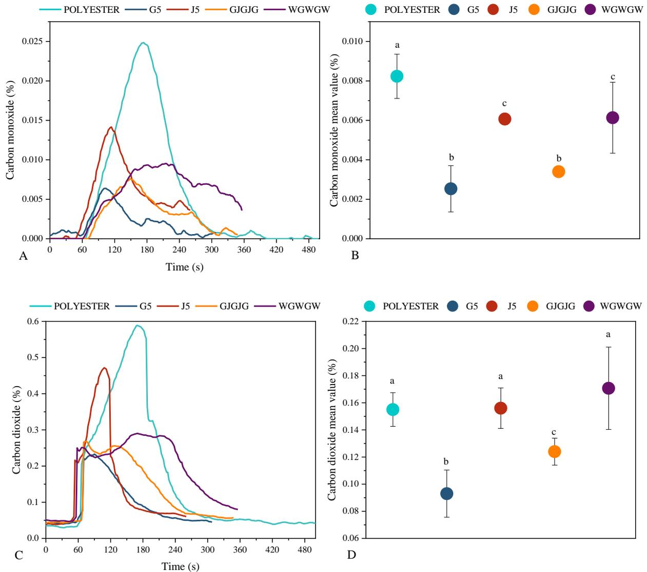
**Figure 7.** Carbon monoxide and carbon dioxide as functions of time for each group analyzed (A,C) and average values for carbon monoxide and carbon dioxide (B,D). Different letters above the errors in each group indicate a statistical difference.
